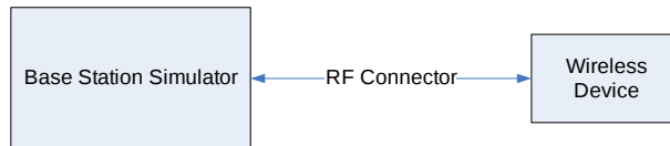
Figure 9-2 Power Measurement Setup
