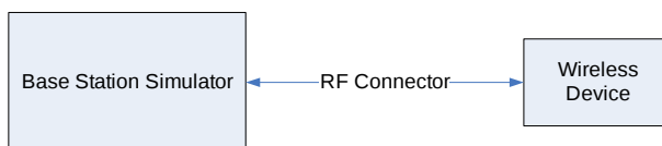
Figure 9-1 Power Measurement Setup
