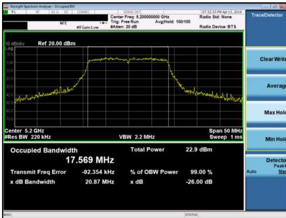
Plot 7-5. 26dB Bandwidth Plot (20MHz BW 802.11n (UNII Band 1) – Ch. 40)
