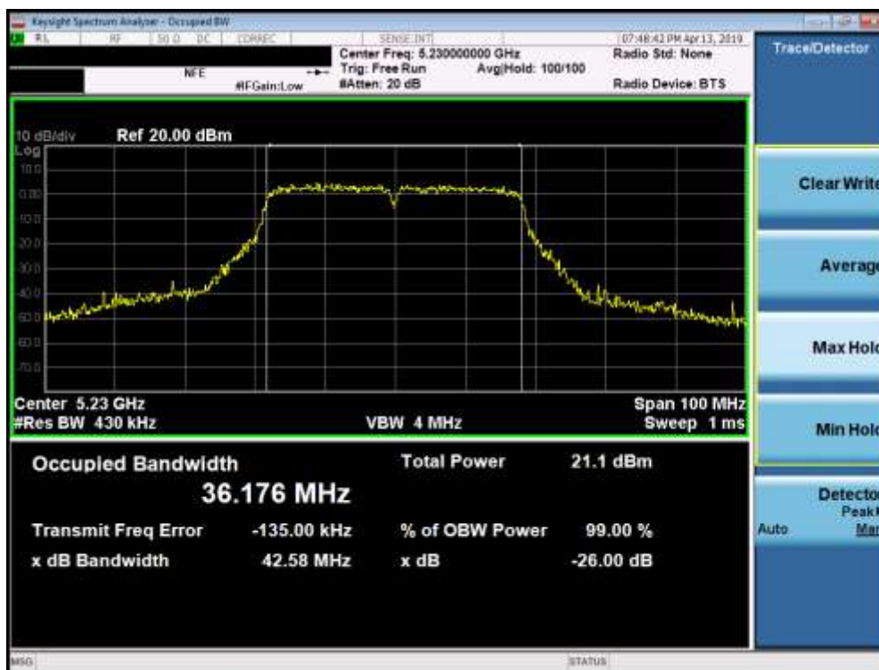
Plot 7-8. 26dB Bandwidth Plot (40MHz BW 802.11n (UNII Band 1) – Ch. 46)
