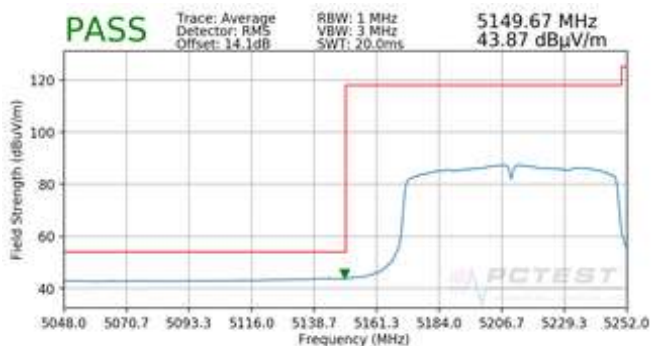
Plot 7-106. Radiated Lower Band Edge Plot (Average – UNII Band 1)
