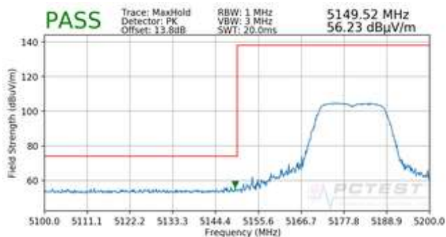
Plot 7-86. Radiated Lower Band Edge Plot (Peak – UNII Band 1)
