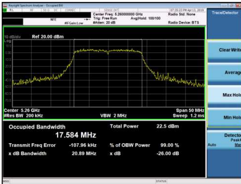
Plot 7-13. 26dB Bandwidth Plot (20MHz BW 802.11n (UNII Band 2A) – Ch. 52)
