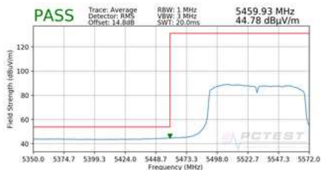
Plot 7-110. Radiated Lower Band Edge Plot (Average – UNII Band 2C)
