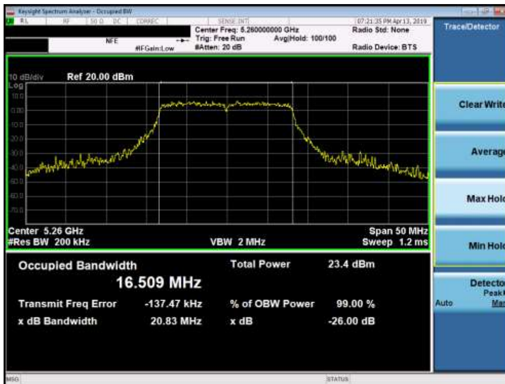
Plot 7-10. 26dB Bandwidth Plot (802.11a (UNII Band 2A) – Ch. 52)
