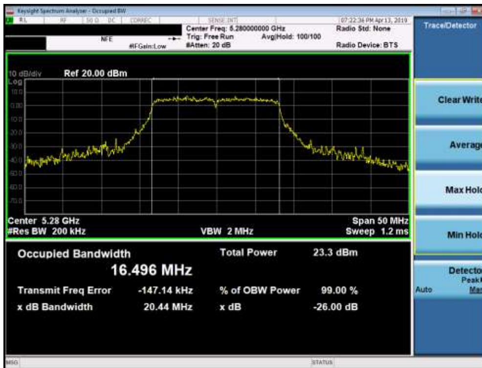
Plot 7-11. 26dB Bandwidth Plot (802.11a (UNII Band 2A) – Ch. 56)
