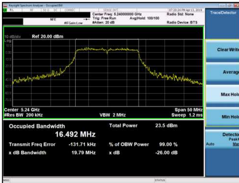
Plot 7-3. 26dB Bandwidth Plot (802.11a (UNII Band 1) – Ch. 48)
