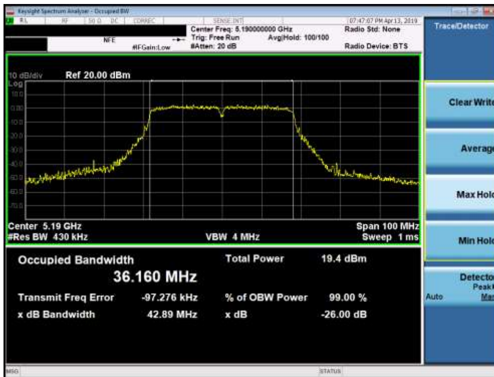
Plot 7-7. 26dB Bandwidth Plot (40MHz BW 802.11n (UNII Band 1) – Ch. 38)
