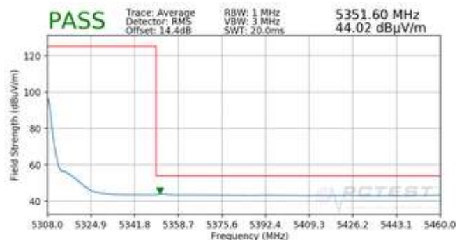
Plot 7-89. Radiated Upper Band Edge Plot (Average – UNII Band 2A)
