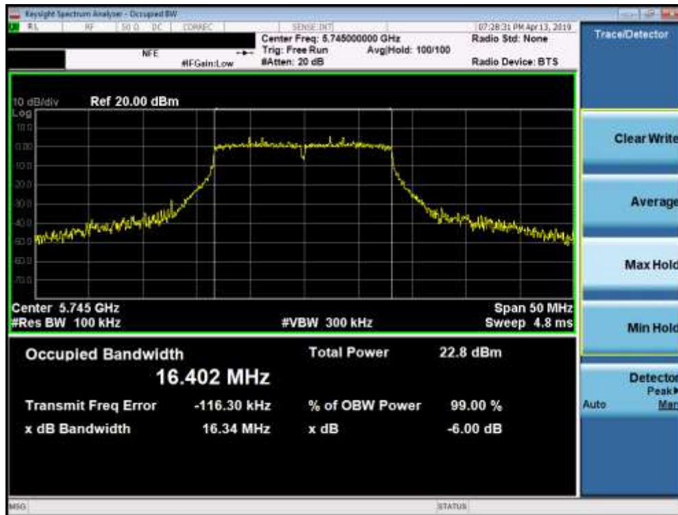
Plot 7-31. 6dB Bandwidth Plot (802.11a (UNII Band 3) – Ch. 149)
