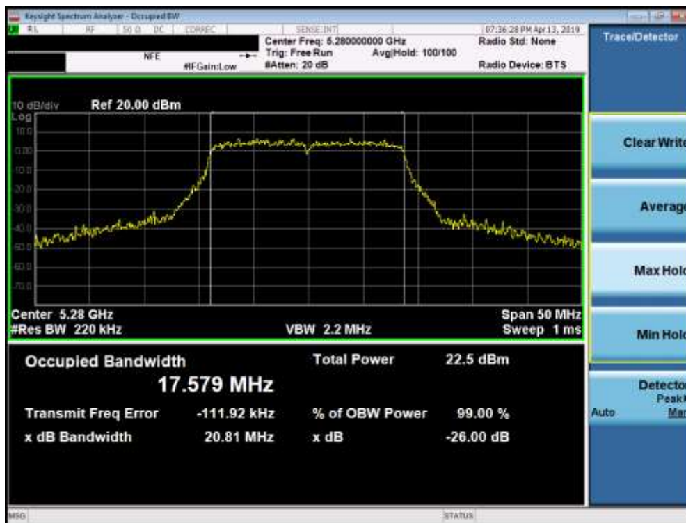
Plot 7-14. 26dB Bandwidth Plot (20MHz BW 802.11n (UNII Band 2A) – Ch. 56)
