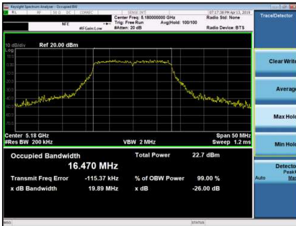
Plot 7-1. 26dB Bandwidth Plot (802.11a (UNII Band 1) – Ch. 36)
