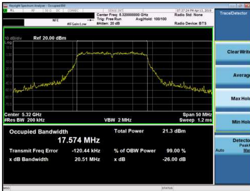
Plot 7-15. 26dB Bandwidth Plot (20MHz BW 802.11n (UNII Band 2A) – Ch. 64)
