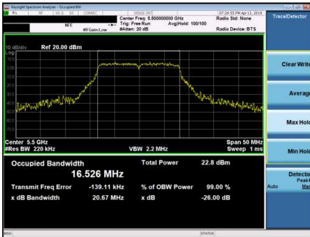
Plot 7-19. 26dB Bandwidth Plot (802.11a (UNII Band 2C) – Ch. 100)
