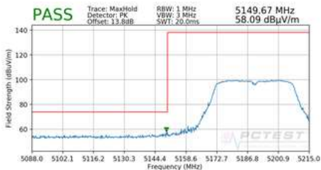
Plot 7-100. Radiated Lower Band Edge Plot (Peak – UNII Band 1)
