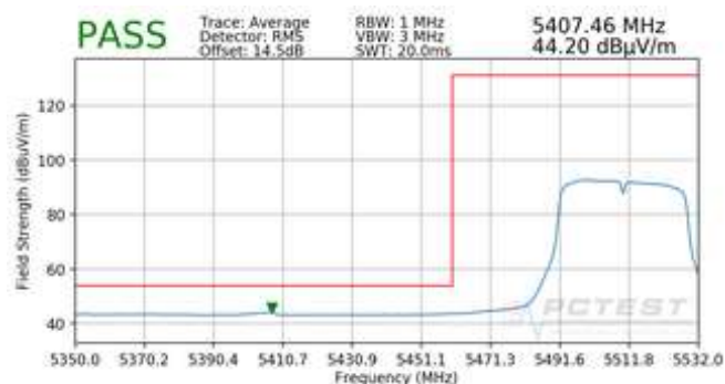
Plot 7-103. Radiated Lower Band Edge Plot (Average – UNII Band 2C)
