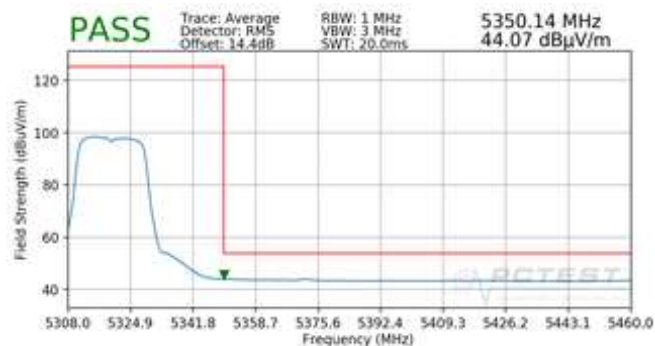
Plot 7-91. Radiated Upper Band Edge Plot (Average – UNII Band 2A)
