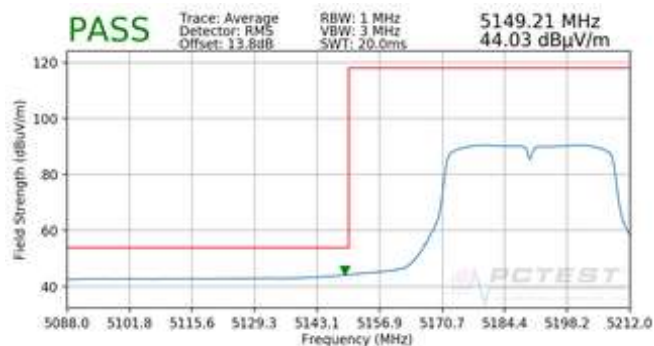
Plot 7-99. Radiated Lower Band Edge Plot (Average – UNII Band 1)
