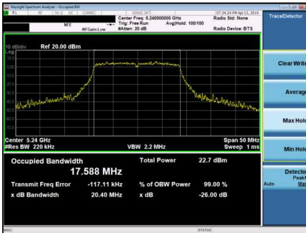
Plot 7-6. 26dB Bandwidth Plot (20MHz BW 802.11n (UNII Band 1) – Ch. 48)
