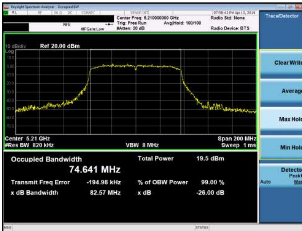
Plot 7-9. 26dB Bandwidth Plot (80MHz BW 802.11ac (UNII Band 1) – Ch. 42)
