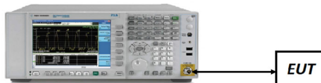
Figure 7-3. Test Instrument & Measurement Setup
