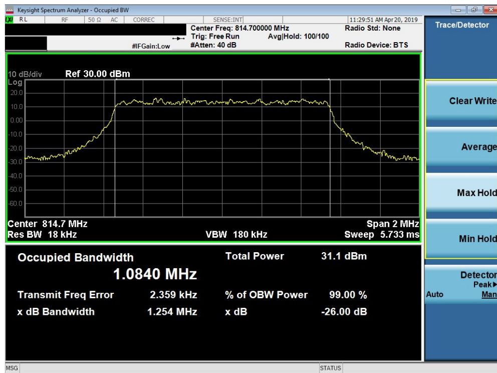
Plot 7-2. Occupied Bandwidth Plot (LTE Band 26, 1.4MHz 16-QAM – RB Size 6– Low Channel)
