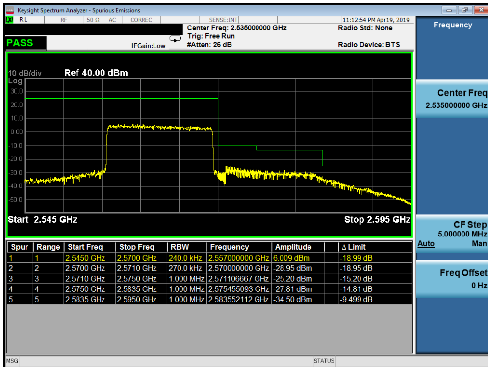
Plot 7-267. Upper ACP Plot (Band 7 - 15.0MHz QPSK - Full RB Configuration)
