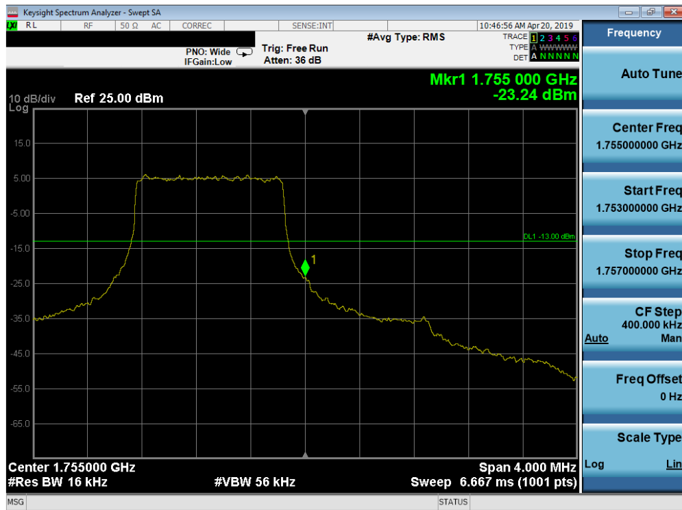
Plot 7-192. Upper Band Edge Plot (Band 4 - 1.4MHz QPSK - Full RB Configuration)
