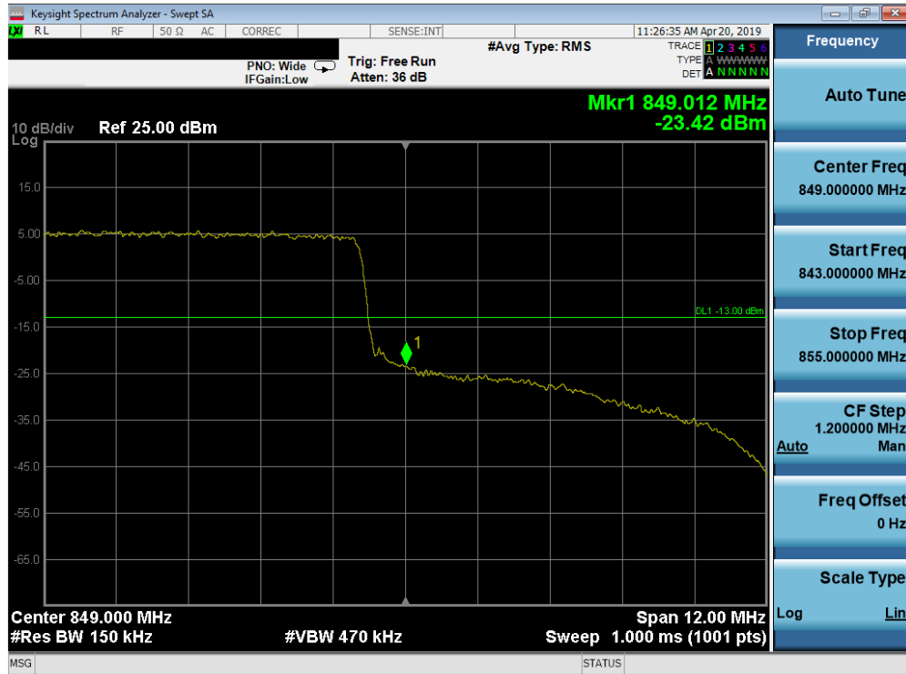
Plot 7-189. Upper Band Edge Plot (Band 26 - 15.0MHz QPSK - Full RB Configuration)
