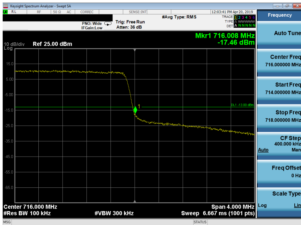
Plot 7-174. Upper Band Edge Plot (Band 12 - 3.0MHz QPSK - Full RB Configuration)
