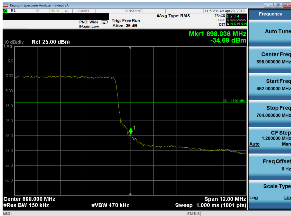
Plot 7-168. Upper Band Edge Plot (Band 71 - 15.0MHz QPSK - Full RB Configuration)
