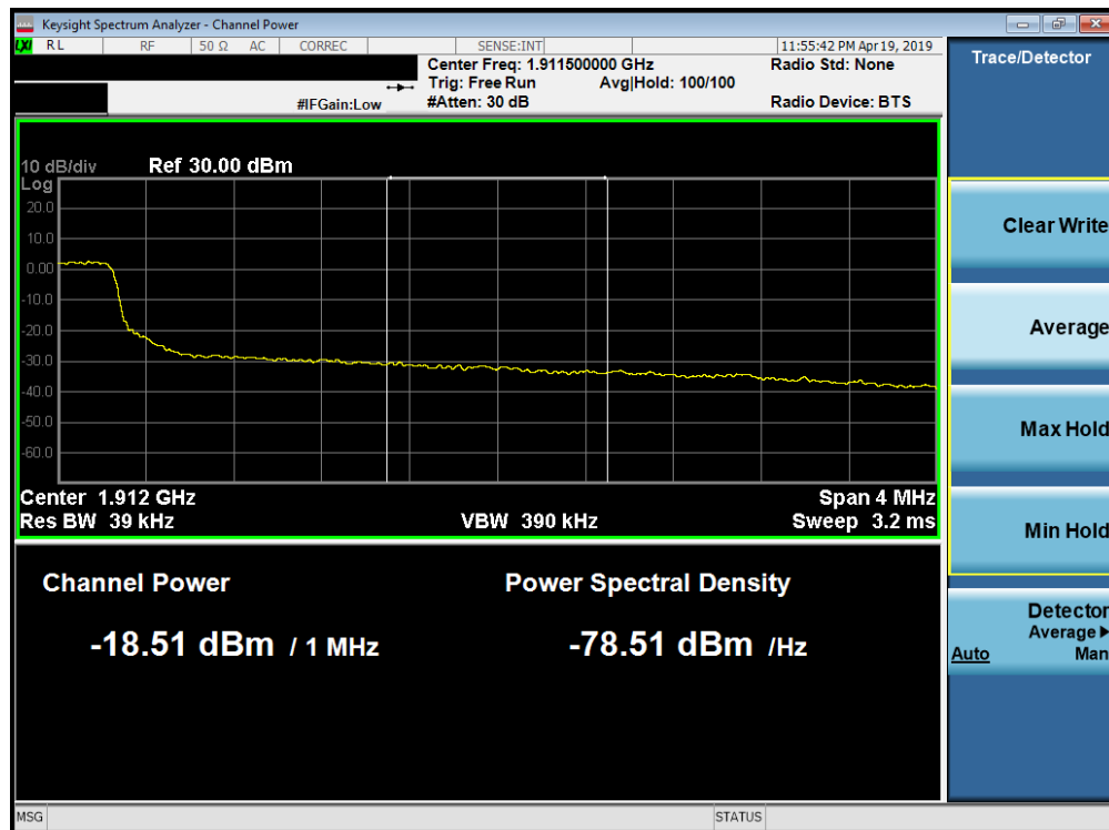
Plot 7-241. Upper Extended Band Edge Plot (Band 2 - 5.0MHz QPSK - Full RB Configuration)
