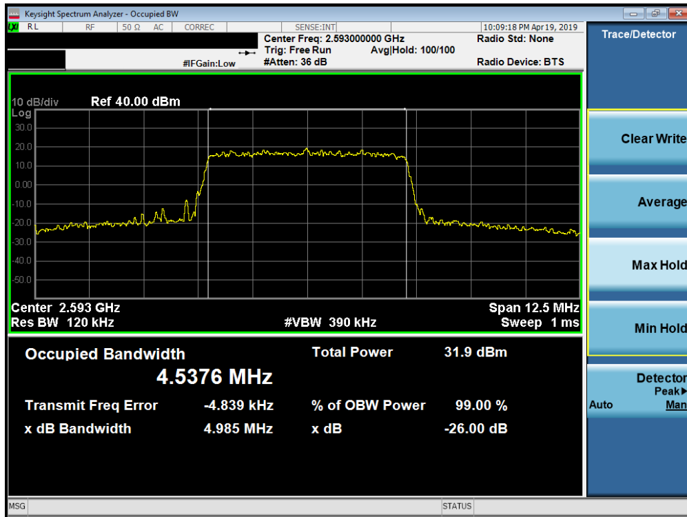
Plot 7-90. Occupied Bandwidth Plot (Band 41 - 5.0MHz 64-QAM - Full RB Configuration)
