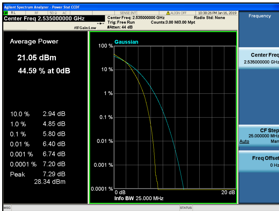
LTE Band 7 / 15 MHz / 16QAM - RB Size 75
