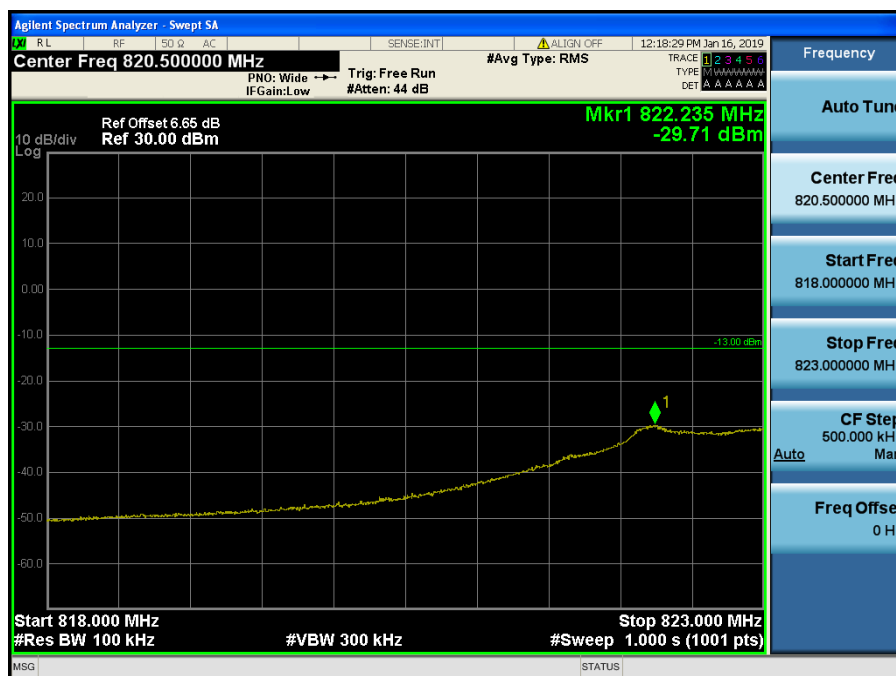
LTE Band 5 / 5MHz / QPSK Size/Offset (12/0)
