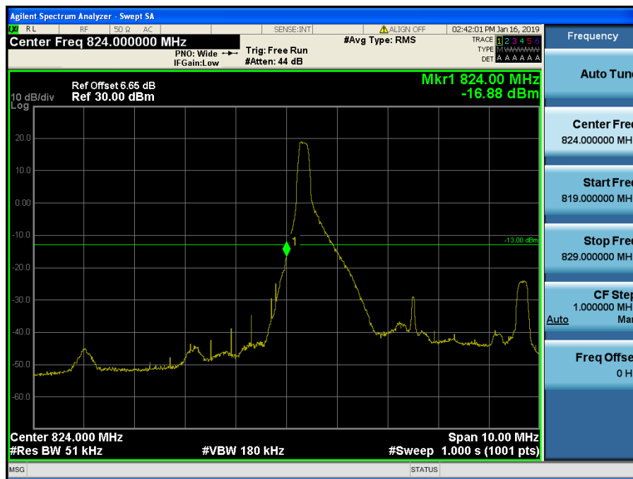
LTE Band 5 / 5MHz / 16QAM Size/Offset (1/0)
