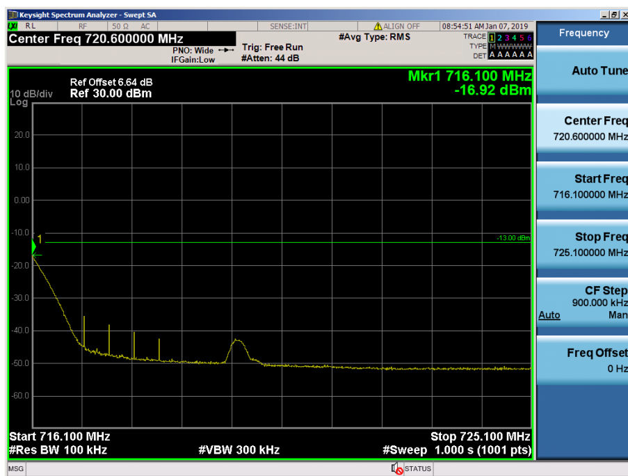
LTE Band 12, 17 / 10MHz / 16QAM - RB Size/Offset (1/49)
