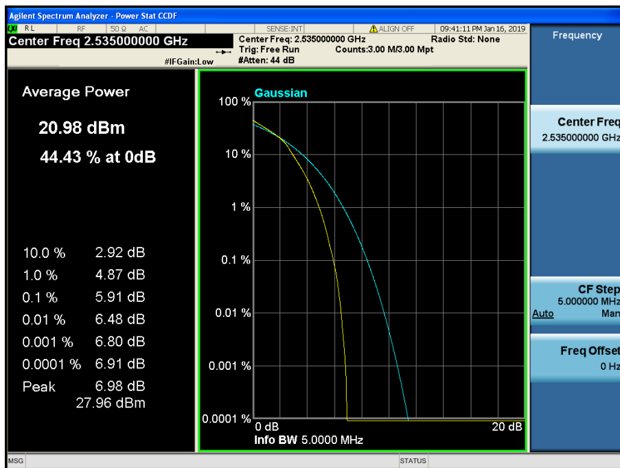
LTE Band 7 / 5 MHz / 16QAM - RB Size 25
