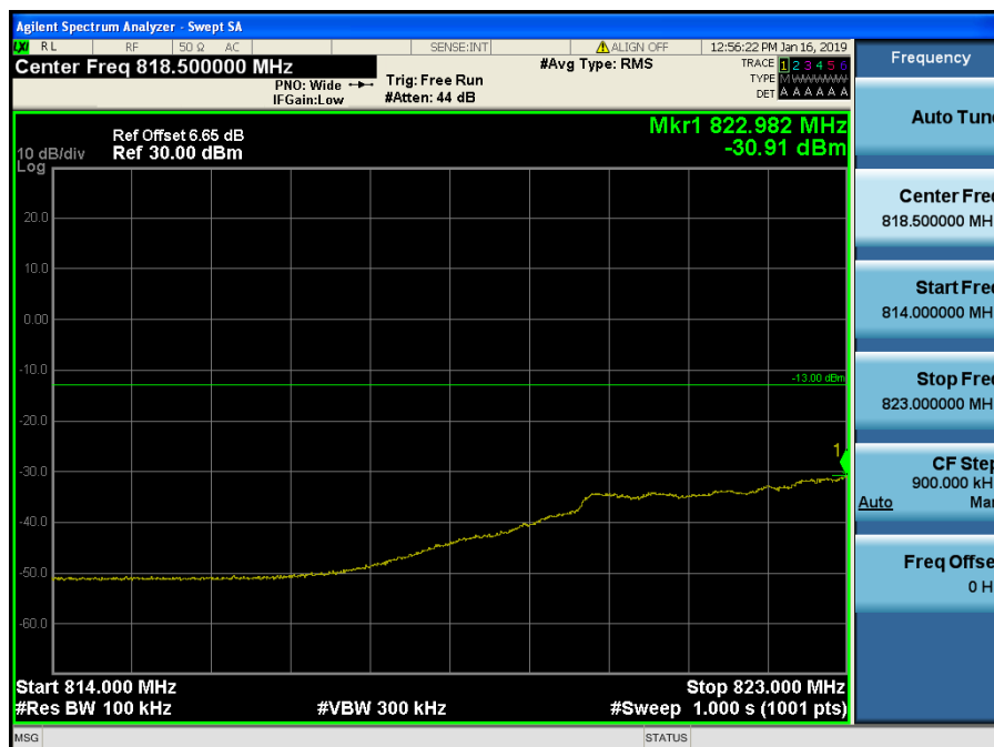
LTE Band 5 / 10MHz / QPSK - RB Size/Offset (25/0)
