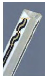
Figure F.2.2 Probe Thick-Film Technique
