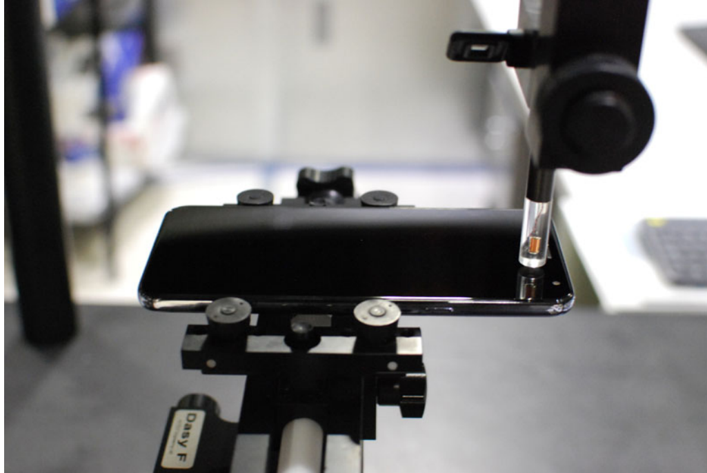
Figure 16-1 Test Setup for Wireless Device
