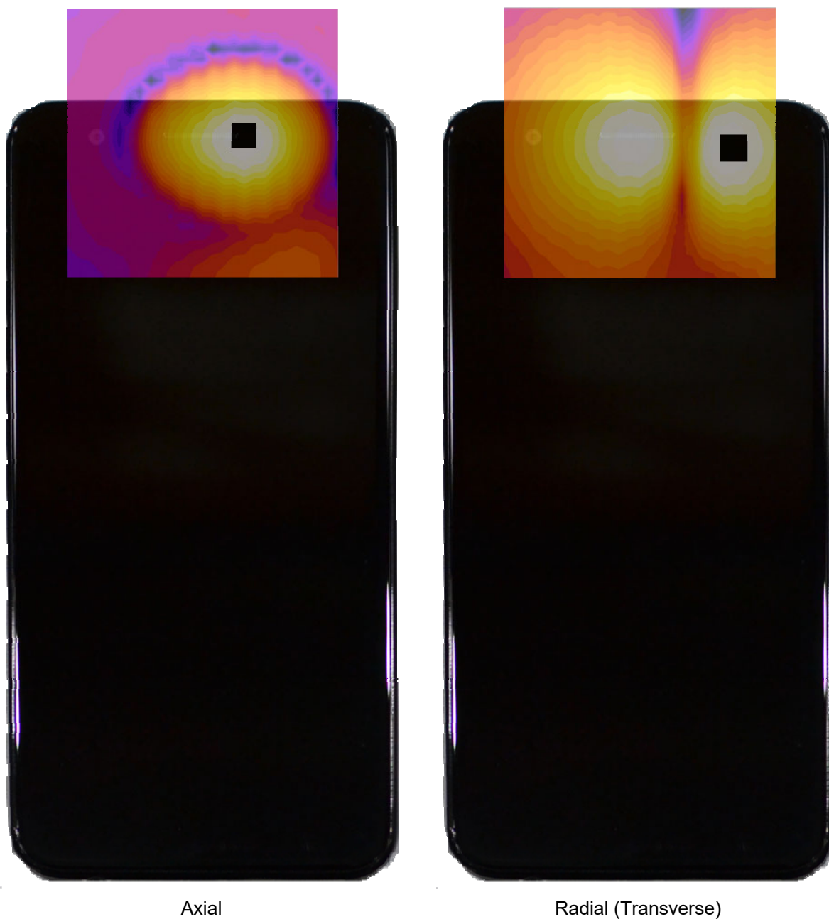
Figure 15-3 T-Coil Scan Overlay Magnetic Field Distributions
