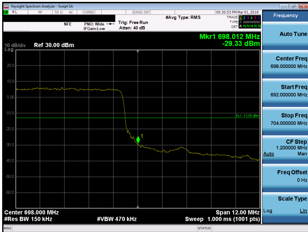
Plot 7-113. Upper Band Edge Plot (Band 71 - 15.0MHz QPSK - Full RB Configuration)
