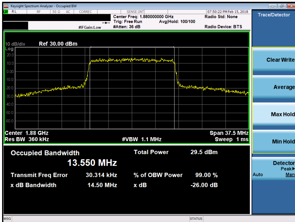
Plot 7-46. Occupied Bandwidth Plot (Band 2 - 15.0MHz 16-QAM - Full RB Configuration)
