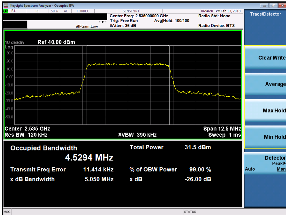
Plot 7-50. Occupied Bandwidth Plot (Band 7 - 5.0MHz 16-QAM - Full RB Configuration)
