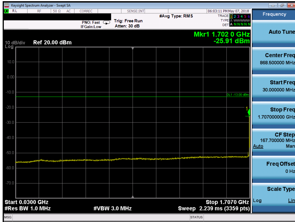
Plot 7-59. Conducted Spurious Plot (Band 4 - 10.0MHz QPSK - RB Size 1, RB Offset 0 - Low Channel)
