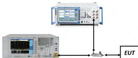
Figure 7-2. Test Instrument & Measurement Setup
