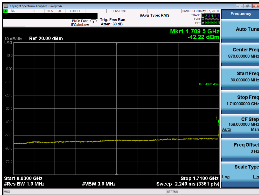
Plot 7-62. Conducted Spurious Plot (Band 4 - 10.0MHz QPSK - RB Size 1, RB Offset 0 - Mid Channel)
