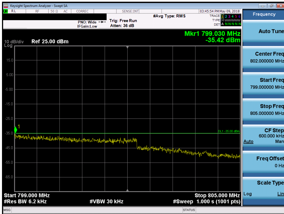
Plot 7-11. Upper Emission Mask Band Edge Plot (LTE B14 - 5MHz QPSK – RB Size 25)
