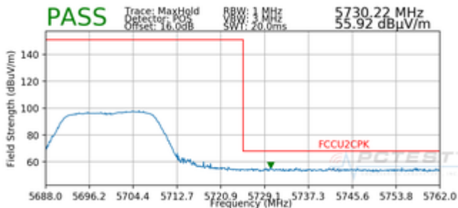
Plot 7-89. Radiated Upper Band Edge Plot SISO ANT1 (Peak – UNII Band 2C)
