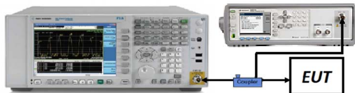
Figure 7-1. Test Instrument & Measurement Setup
