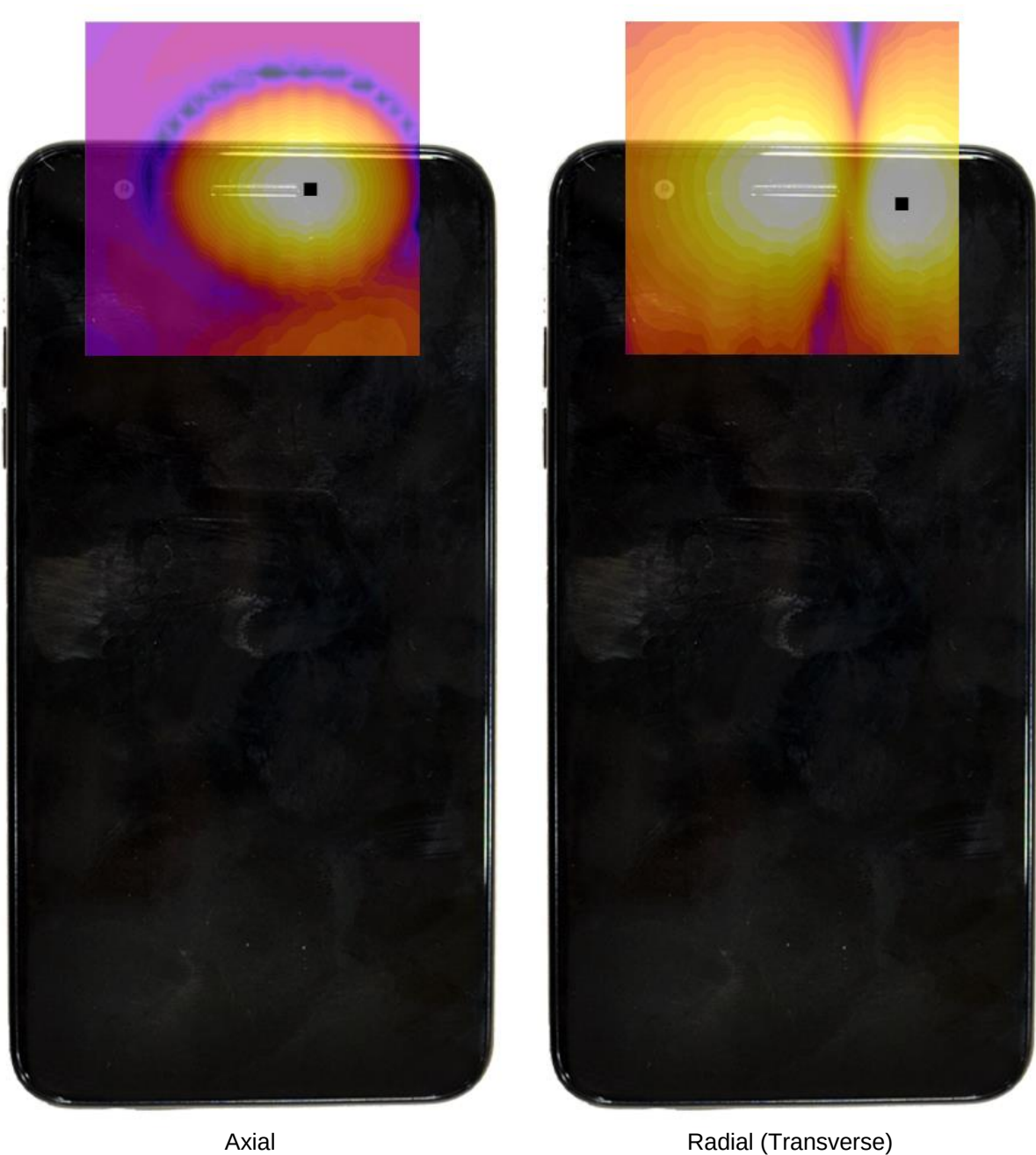
Figure 16-3 T-Coil Scan Overlay Magnetic Field Distributions
