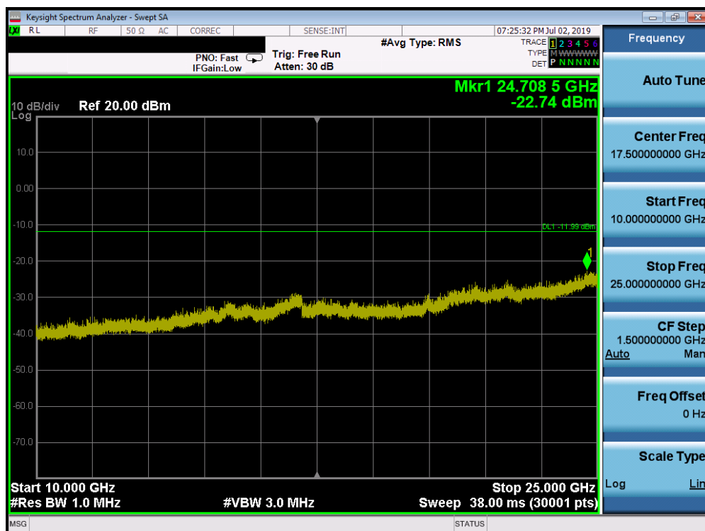
Plot 7-41. Conducted Spurious Plot (Bluetooth, 1Mbps – Ch. 78)
