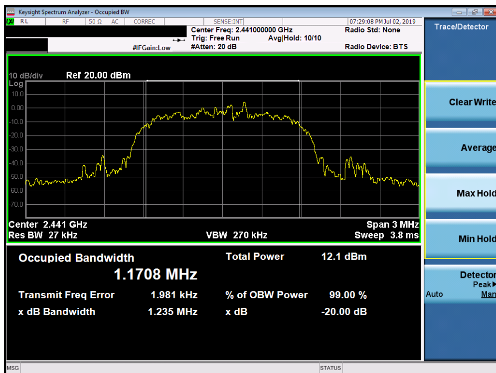
Plot 7-5. 20dB Bandwidth Plot (Bluetooth, 2Mbps – Ch. 39)
