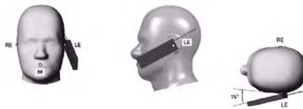
Figure 5.3 Front, Side and Top View of Ear/15° Position
