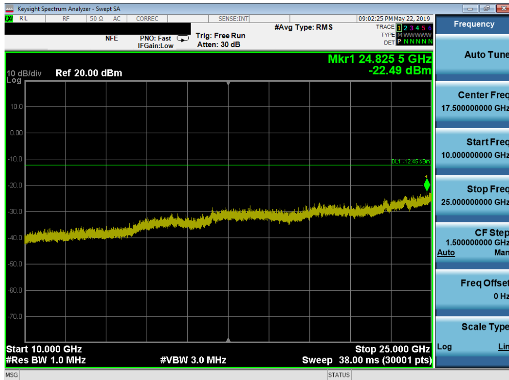
Plot 7-41. Conducted Spurious Plot (Bluetooth, 3Mbps – Ch. 78)
