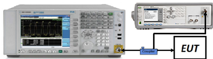
Figure 7-6. Test Instrument & Measurement Setup
