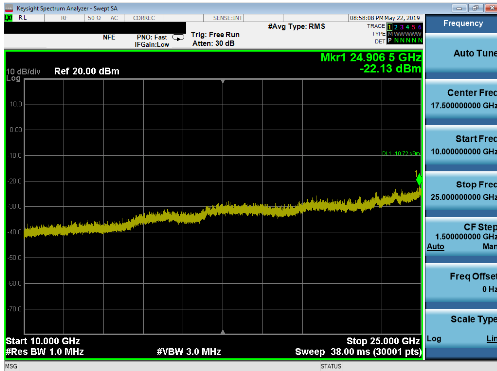
Plot 7-39. Conducted Spurious Plot (Bluetooth, 3Mbps – Ch. 39)
