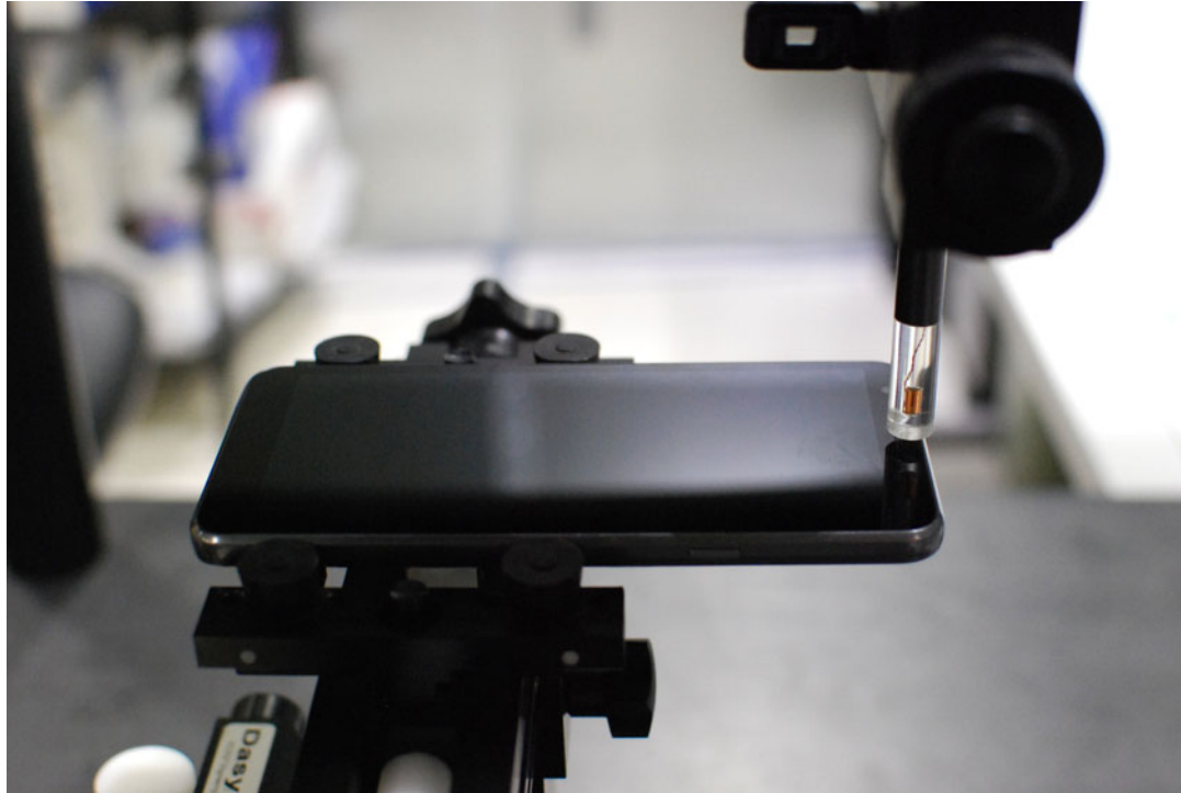
Figure 16-1 Test Setup for Wireless Device
