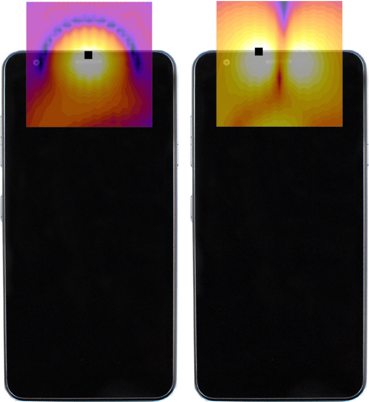
Figure 16-3 T-Coil Scan Overlay Magnetic Field Distributions
