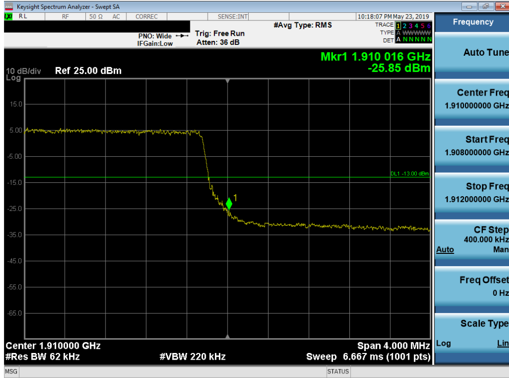
Plot 7-128. Upper Band Edge Plot (Band 2 - 5.0MHz QPSK - Full RB Configuration)
