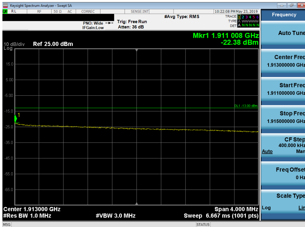
Plot 7-133. Upper Extended Band Edge Plot (Band 2 - 10.0MHz QPSK - Full RB Configuration)
