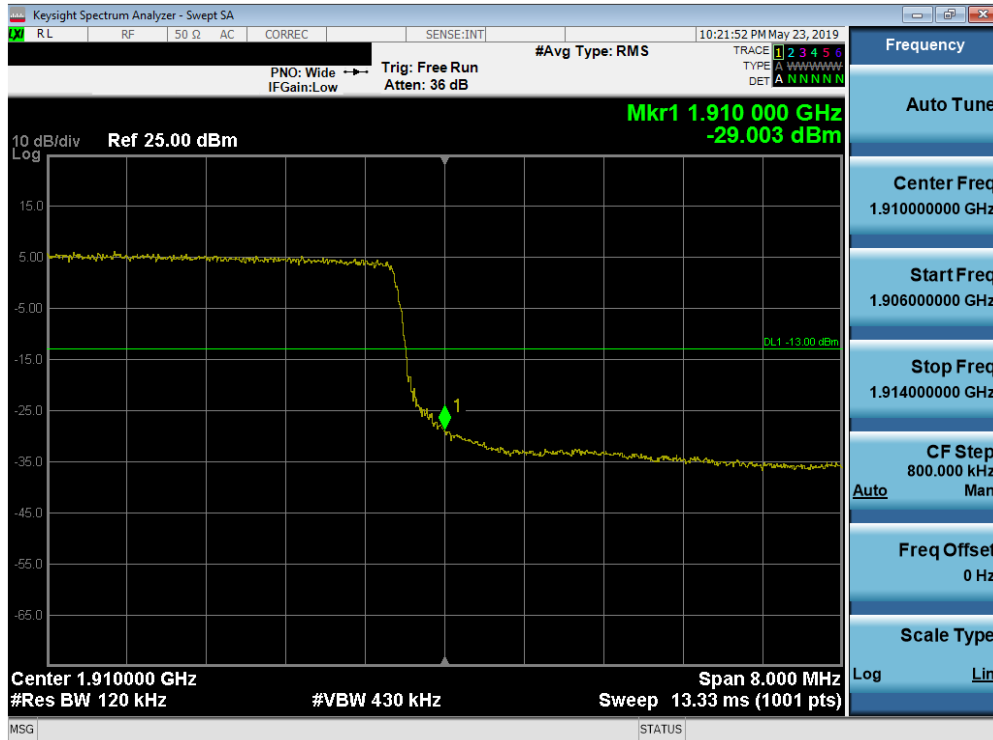
Plot 7-132. Upper Band Edge Plot (Band 2 - 10.0MHz QPSK - Full RB Configuration)
