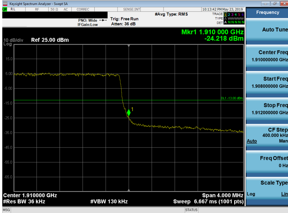
Plot 7-124. Upper Band Edge Plot (Band 2 - 3.0MHz QPSK - Full RB Configuration)
