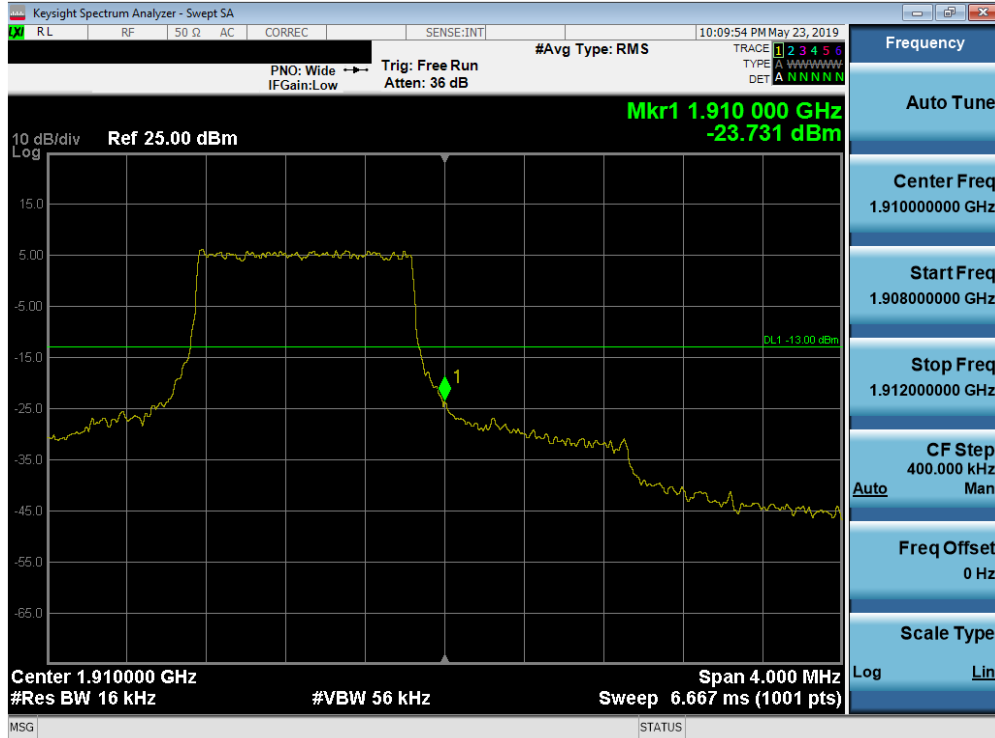
Plot 7-120. Upper Band Edge Plot (Band 2 - 1.4MHz QPSK - Full RB Configuration)
