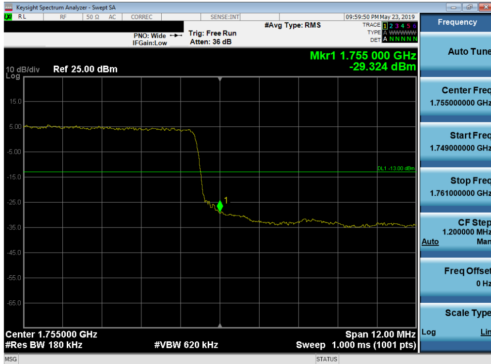
Plot 7-112. Upper Band Edge Plot (Band 4 - 15.0MHz QPSK - Full RB Configuration)
