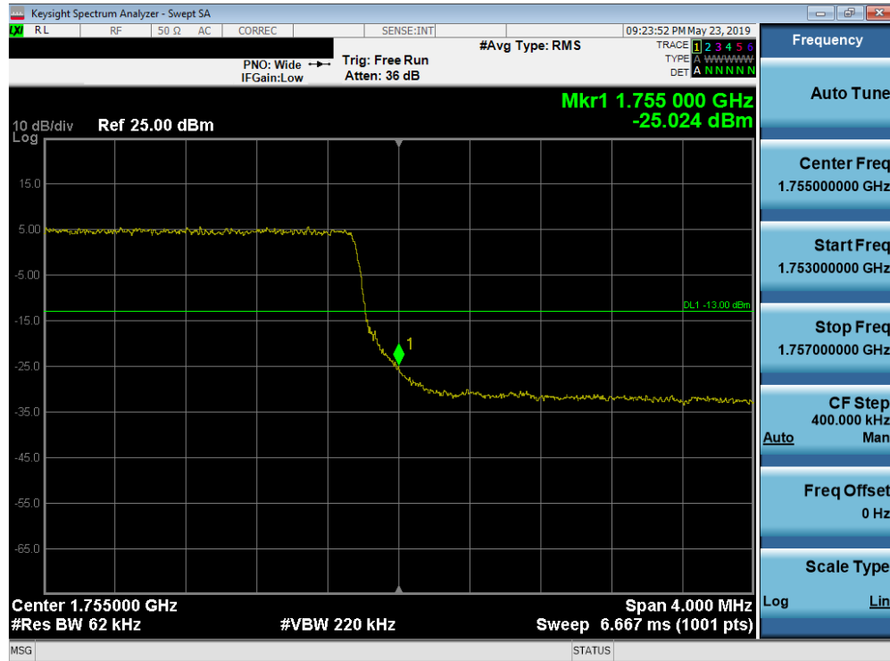
Plot 7-104. Upper Band Edge Plot (Band 4 - 5.0MHz QPSK - Full RB Configuration)
