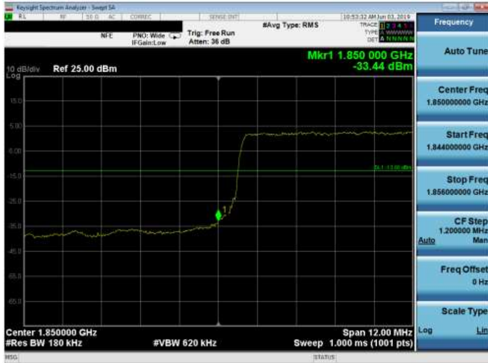
Plot 7-133. Lower Band Edge Plot (Band 2 - 15.0MHz QPSK - Full RB Configuration)
