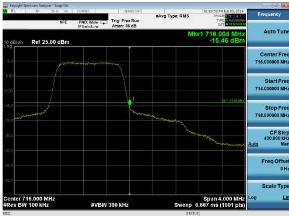
Plot 7-78. Upper Band Edge Plot (Band 12 - 1.4MHz QPSK - Full RB Configuration)
