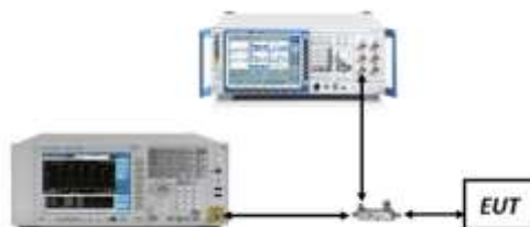
Figure 7-3. Test Instrument & Measurement Setup
