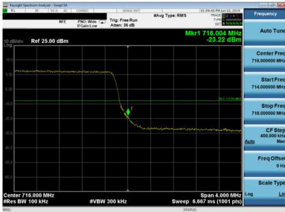
Plot 7-82. Upper Band Edge Plot (Band 12 - 5.0MHz QPSK - Full RB Configuration)
