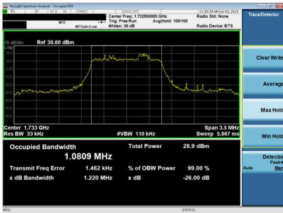
Plot 7-17. Occupied Bandwidth Plot (Band 4 - 1.4MHz QPSK - Full RB Configuration)
