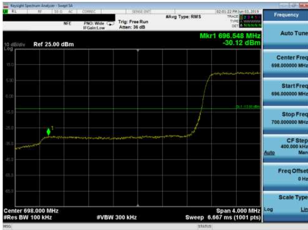
Plot 7-79. Lower Band Edge Plot (Band 12 - 3.0MHz QPSK - Full RB Configuration)
