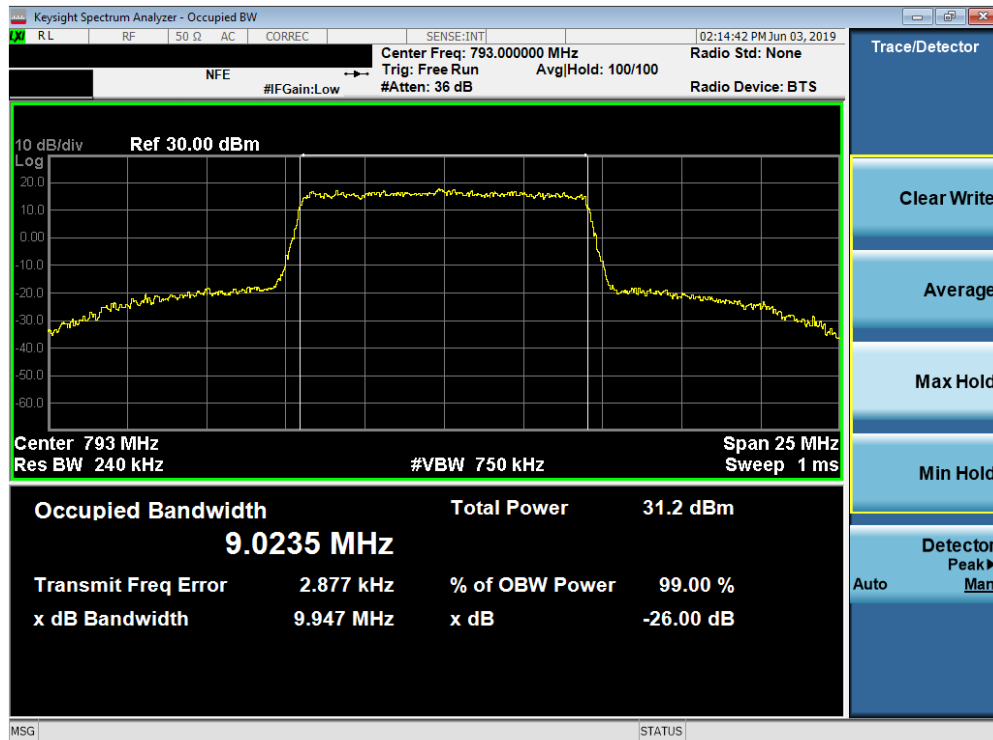
Plot 7-4. Occupied Bandwidth Plot (LTE Band 14, 10MHz 16-QAM – RB Size 50)
