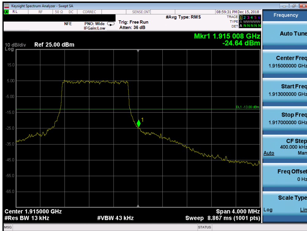
Plot 7-121. Upper Band Edge Plot (Band 25 - 1.4MHz QPSK - Full RB Configuration)
