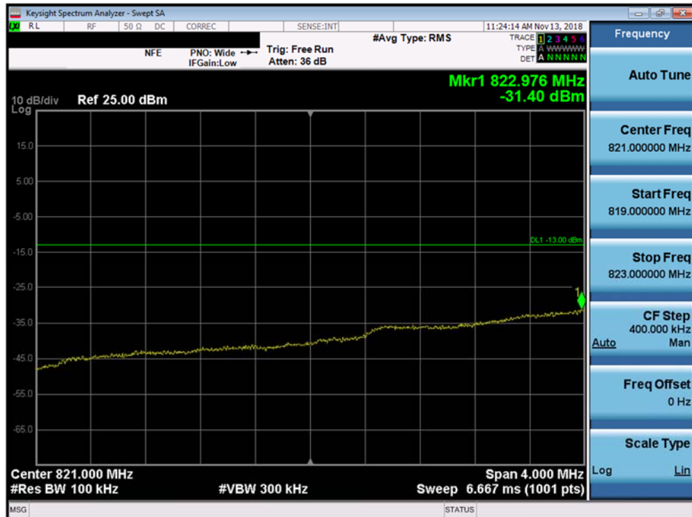
Plot 7-46. Lower Extended Band Edge Plot (Band 26 - 3.0MHz QPSK - Full RB Configuration)
