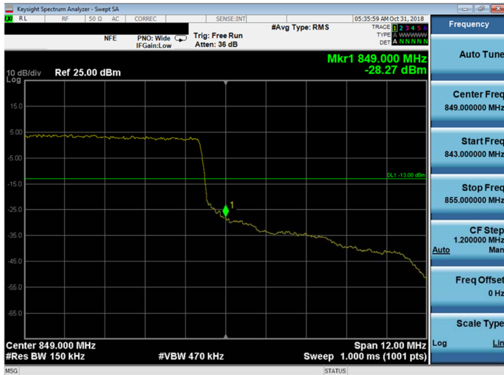
Plot 7-54. Upper Band Edge Plot (Band 26 - 15.0MHz QPSK - Full RB Configuration)
