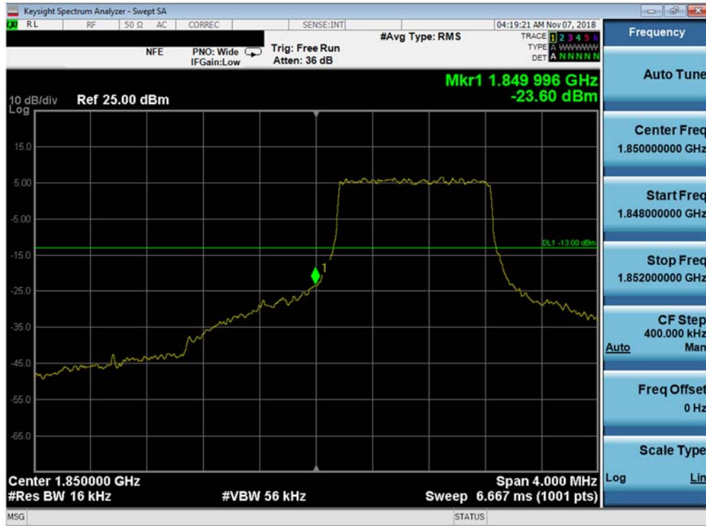
Plot 7-55. Lower Band Edge Plot (Band 25 - 1.4MHz QPSK - Full RB Configuration)
