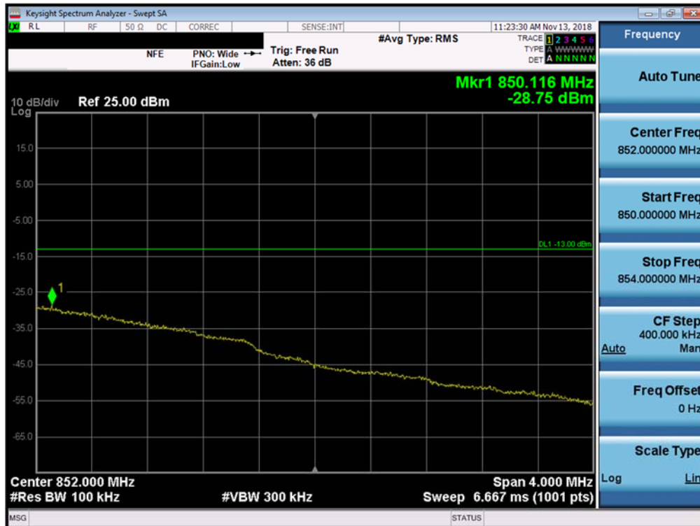
Plot 7-48. Upper Extended Band Band Edge Plot (Band 26 - 3.0MHz QPSK - Full RB Configuration)
