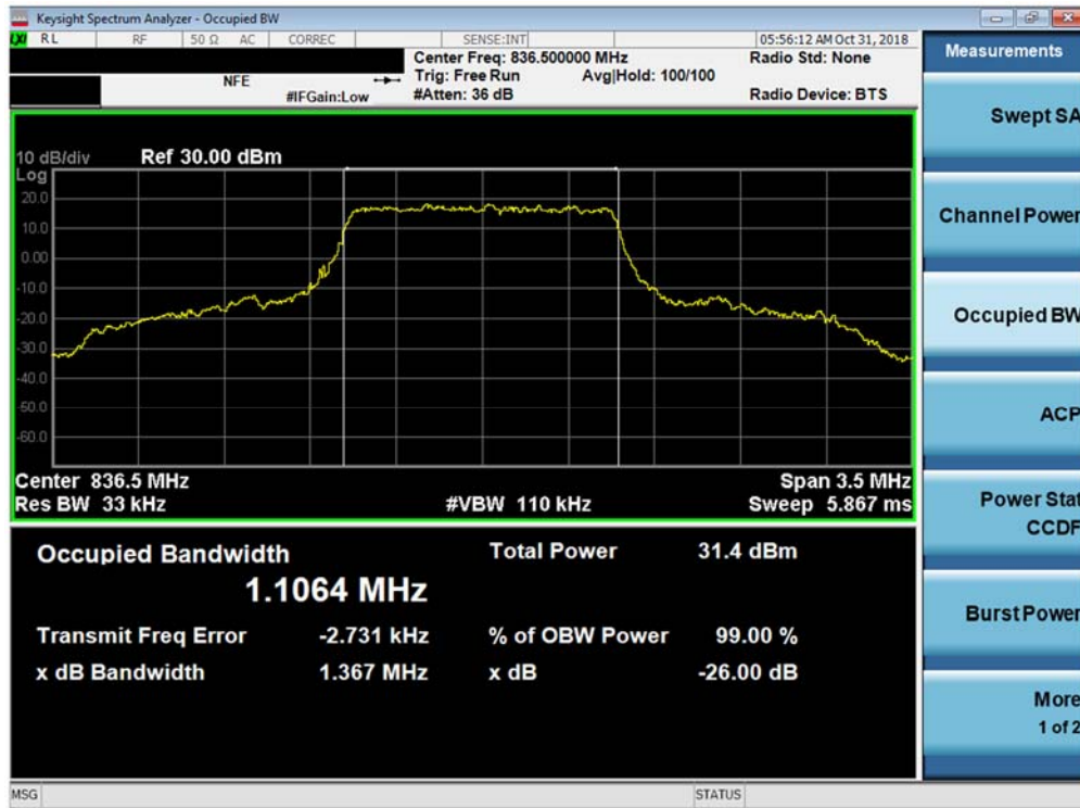
Plot 7-1. Occupied Bandwidth Plot (Band 26 - 1.4MHz QPSK - Full RB Configuration)
