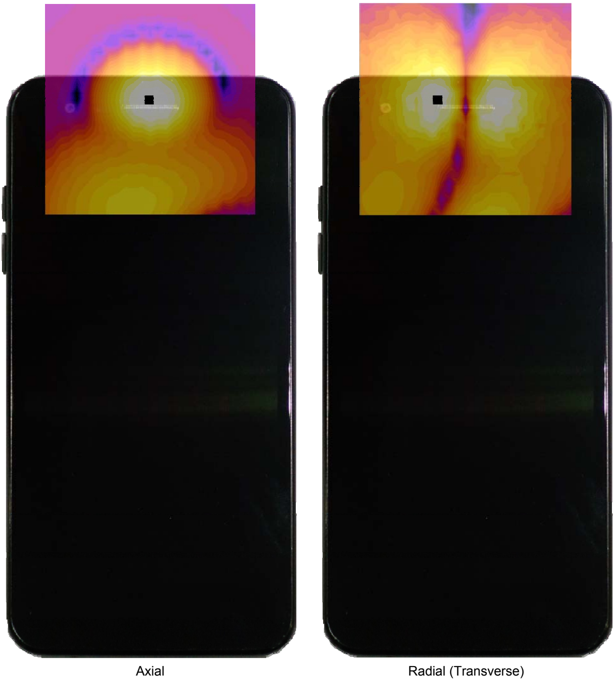
Figure 16-3 T-Coil Scan Overlay Magnetic Field Distributions
