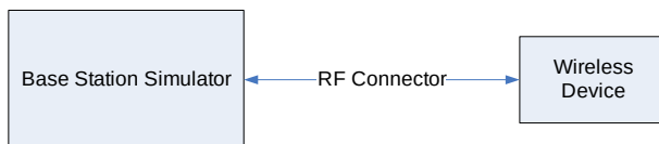
Figure 9-1 Power Measurement Setup
