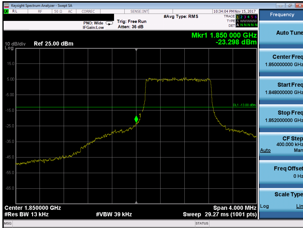
Plot 7-117. Lower Band Edge Plot (Band 2 - 1.4MHz QPSK - Full RB Configuration)
