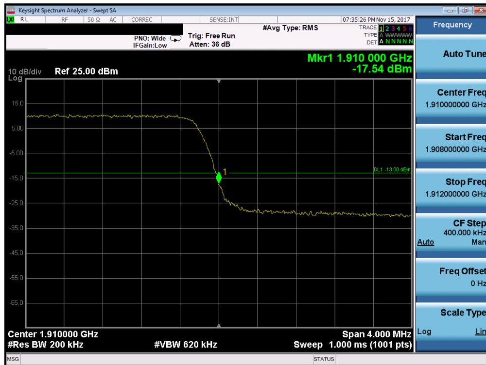
Plot 7-127. Upper Band Edge Plot (Band 2 - 5.0MHz QPSK - Full RB Configuration)
