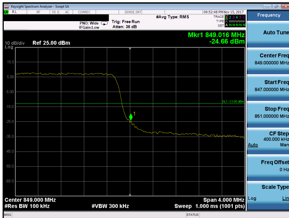
Plot 7-90. Upper Band Edge Plot (Band 5 – 5.0MHz QPSK - Full RB Configuration)
