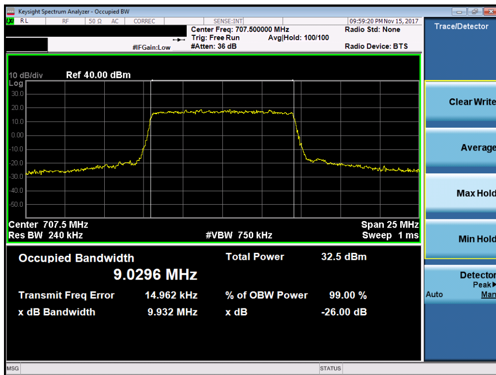
Plot 7-7. Occupied Bandwidth Plot (Band 12 - 10.0MHz QPSK - Full RB Configuration)
