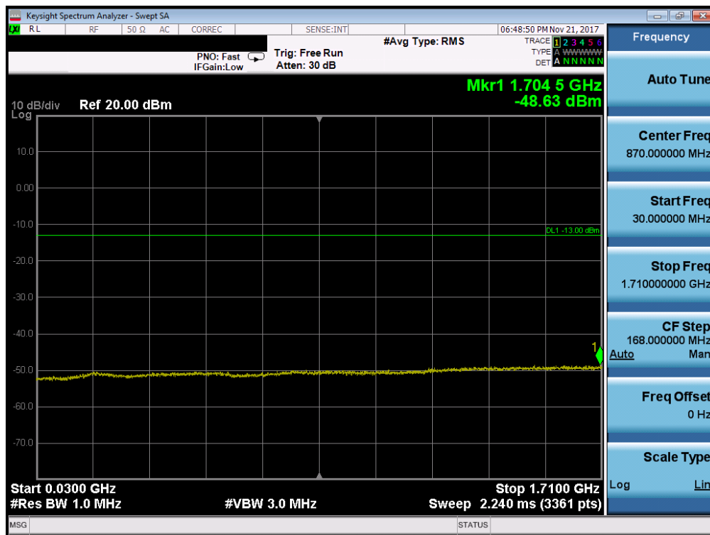
Plot 7-62. Conducted Spurious Plot (Band 4 - 15.0MHz QPSK - RB Size 1, RB Offset 0 - Mid Channel)
