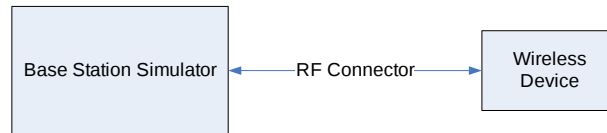
Figure 9-2 Power Measurement Setup
