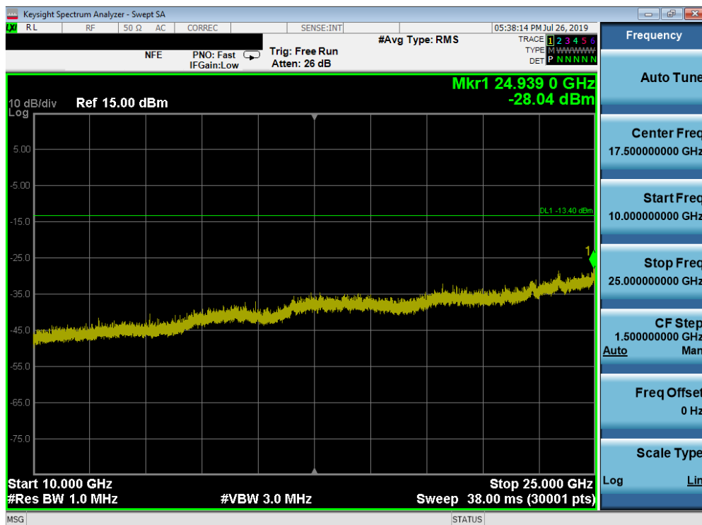
Plot 7-39. Conducted Spurious Plot (Bluetooth, 1Mbps – Ch. 39)
