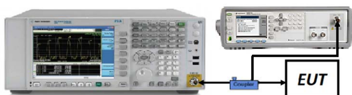
Figure 7-5. Test Instrument & Measurement Setup
