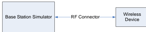
Figure 9-1 Power Measurement Setup
