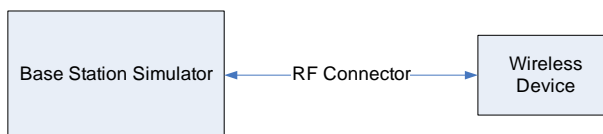
Figure 9-2 Power Measurement Setup
