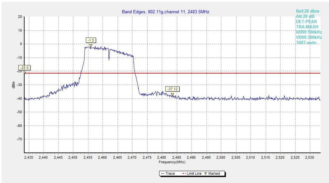
Fig.A.5.4 Band Edges (802.11g, Ch 11)
