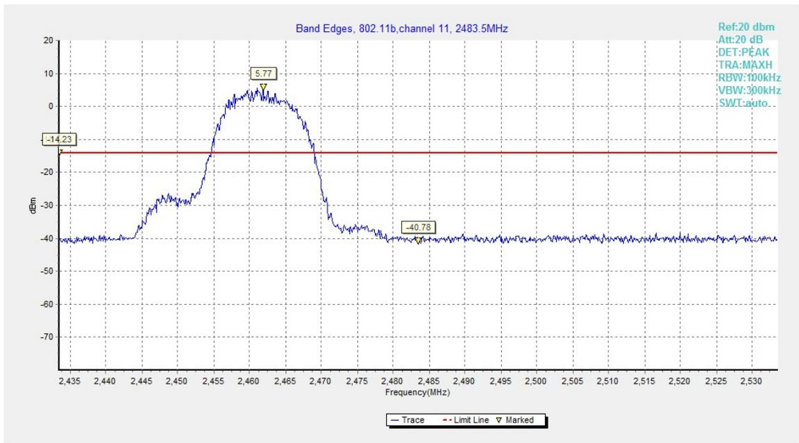
Fig.A.5.2 Band Edges (802.11b, Ch 11)
