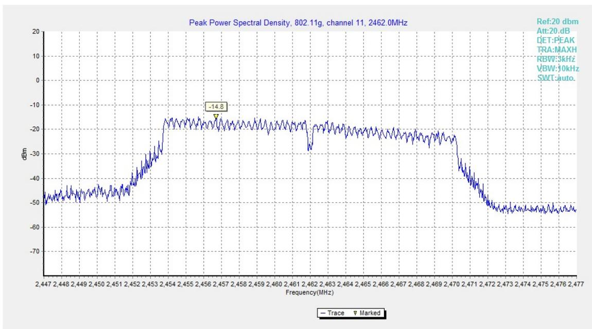
**Fig.A.3.6 Power Spectral Density (802.11g, Ch 11)**
