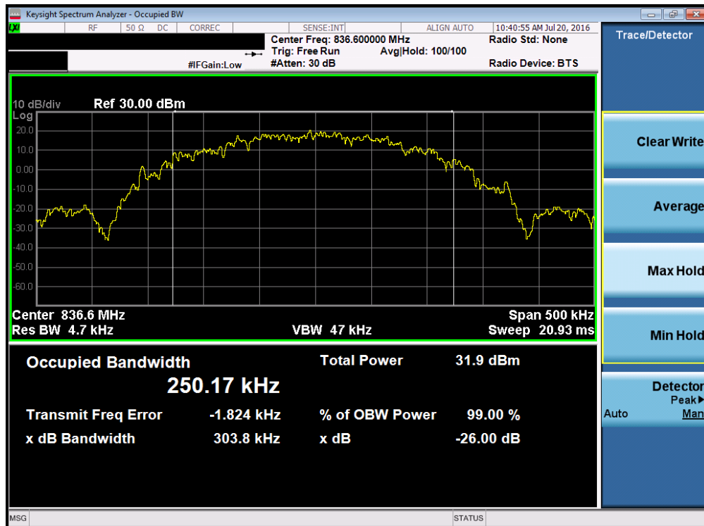
Plot 7-2. Occupied Bandwidth Plot (EDGE850 Mode – Ch. 190)
