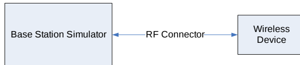
Figure 9-4 Power Measurement Setup
