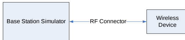
Figure 9-3 Power Measurement Setup
