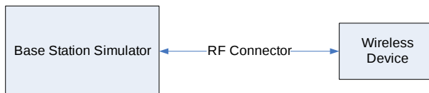
Figure 9-1 Power Measurement Setup
