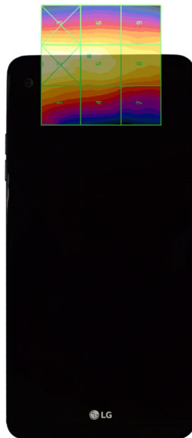
Figure 17-4 E-Field WD Scan overlay
