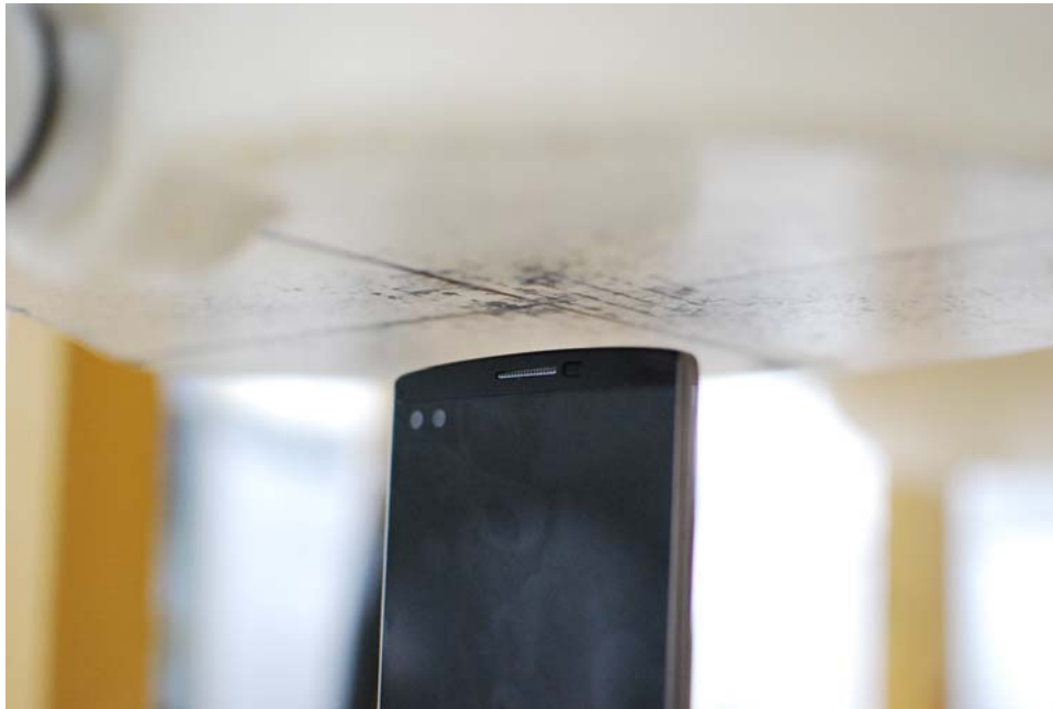
SAR Test Setup Photo 14: Top Edge, Standard Cover at 10 mm
