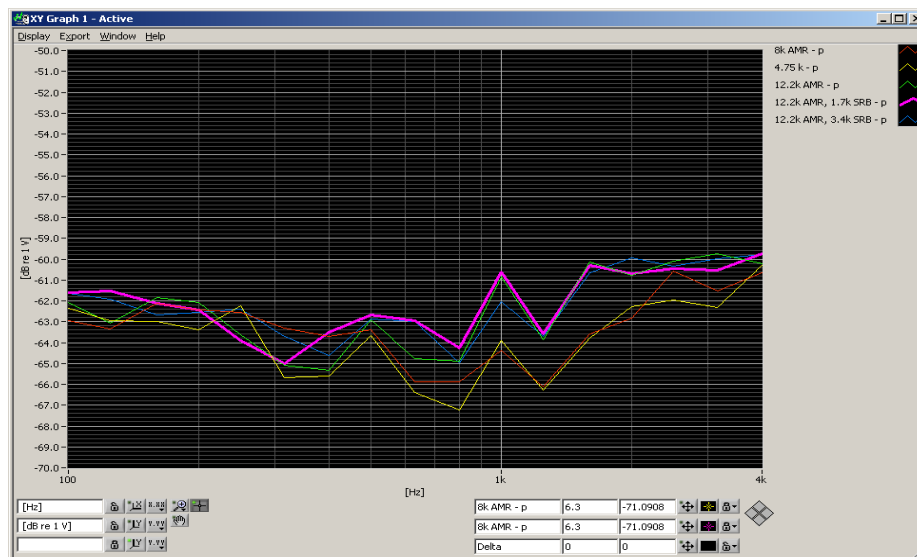
Figure 7-2 UMTS Audio Band Magnetic Noise
