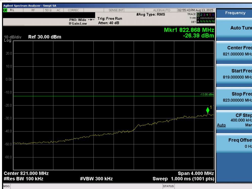
Plot 6-103. Lower Extended Band Edge Plot (Band 5 – 3.0MHz QPSK – RB Size 15)
