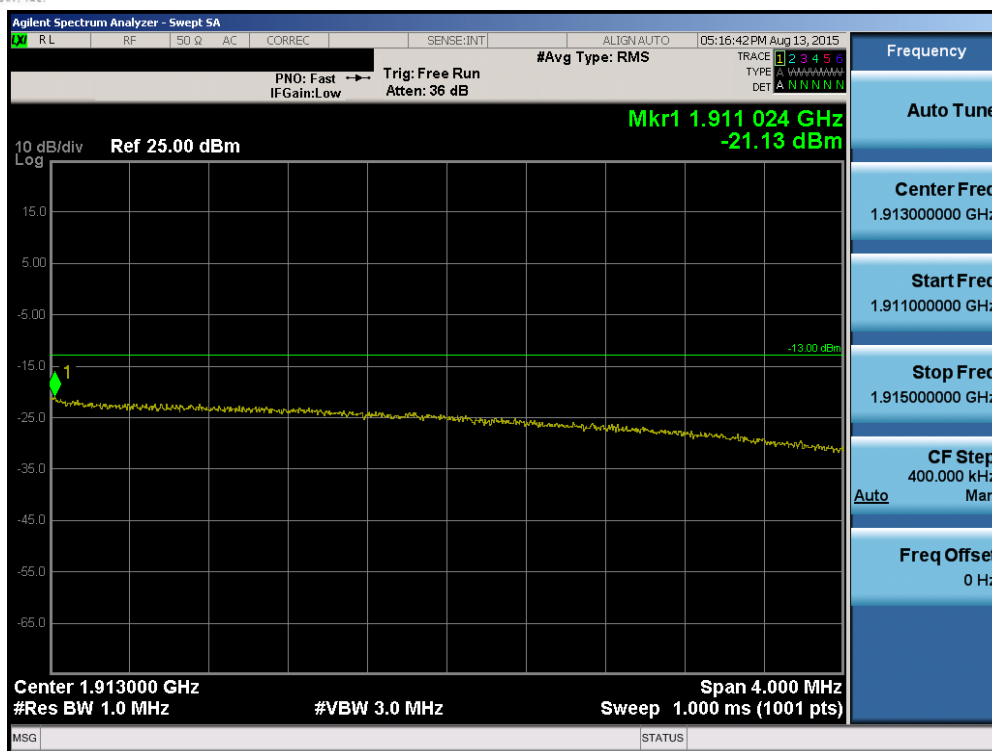
Plot 6-151. Upper Extended Band Edge Plot (Band 2 - 10.0MHz QPSK - RB Size 50)
