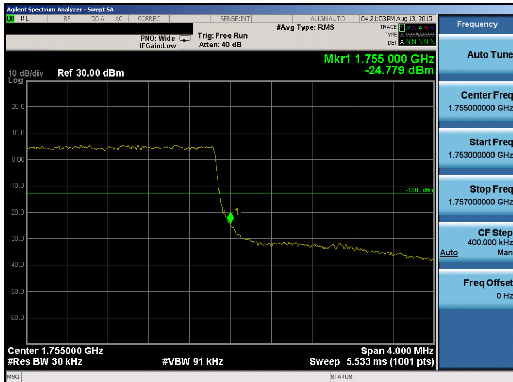
Plot 6-118. Upper Band Edge Plot (Band 4 – 3.0MHz QPSK – RB Size 15)
