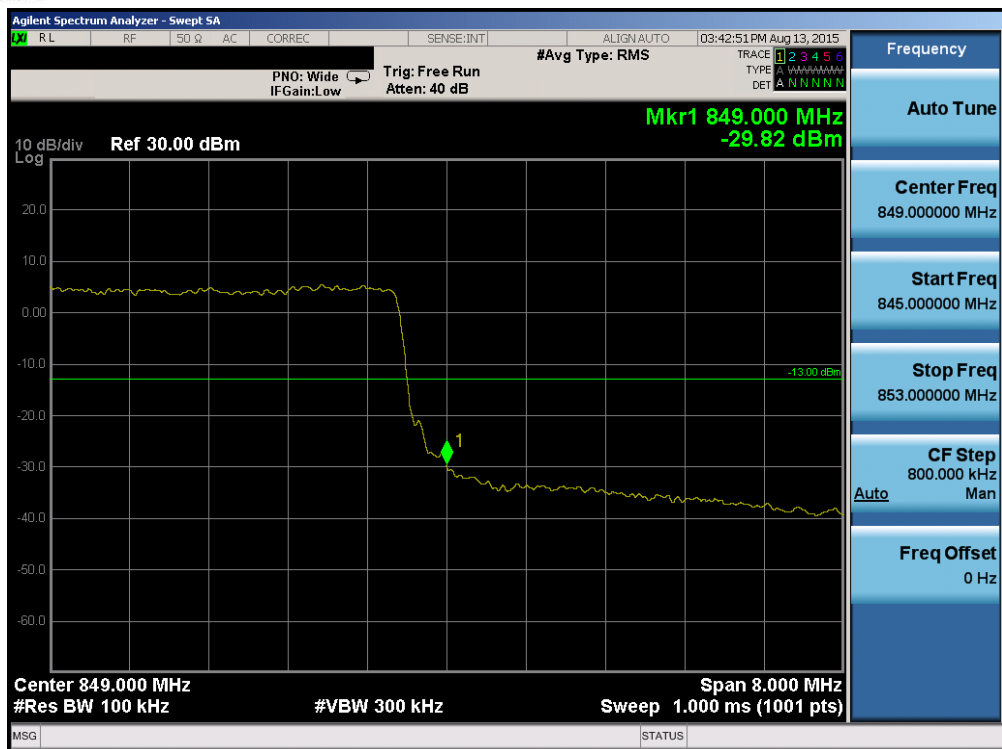
Plot 6-111. Upper Band Edge Plot (Band 5 - 10.0MHz QPSK - RB Size 50)
