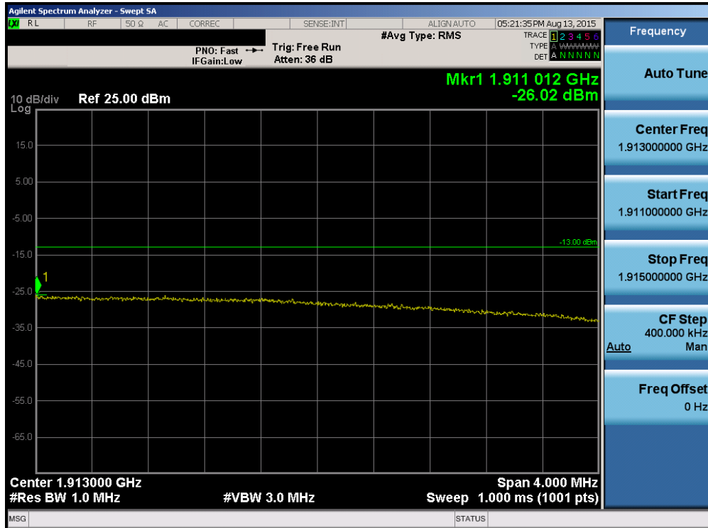
Plot 6-159. Upper Extended Band Edge Plot (Band 2 - 20.0MHz QPSK - RB Size 100)
