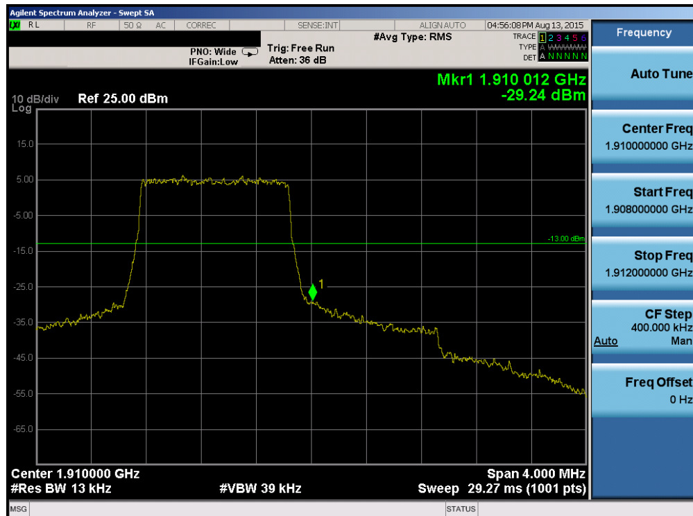
Plot 6-138. Upper Band Edge Plot (Band 2 – 1.4MHz QPSK – RB Size 6)
