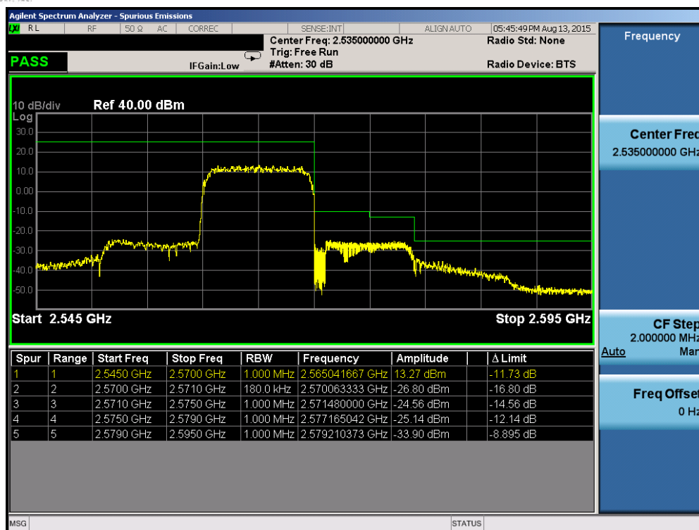
Plot 6-163. Upper ACP Plot (Band 7 – 10.0MHz QPSK – RB Size 50)
