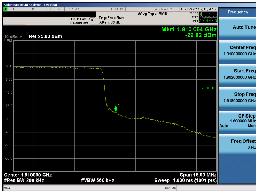
Plot 6-158. Upper Band Edge Plot (Band 2 – 20.0MHz QPSK – RB Size 100)
