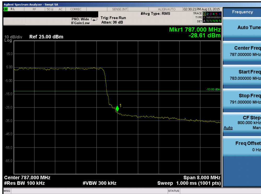
Plot 6-96. Upper Band Edge Plot (Band 13 - 10.0MHz QPSK - RB Size 50)
