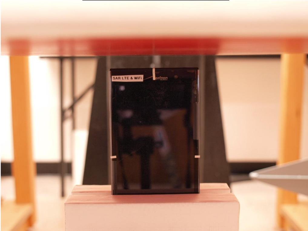
Hotspot – Edge 1 with 10 mm Separation with Wireless Charging Battery Cover
