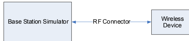
Figure 9-1 Power Measurement Setup
