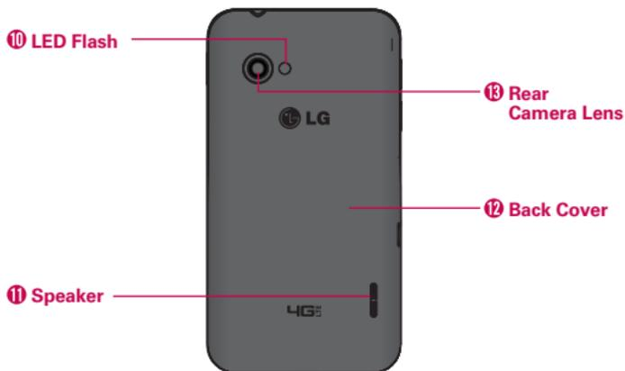
10. **LED Flash** Brightens up the captured image or recorded video when you turn on the flash.
