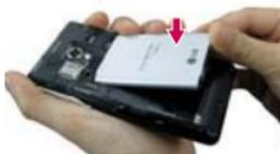
2. Insert the battery, making sure to align the gold contacts. Press down gently to secure the battery.
