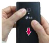
3. Place the cover over the back of the phone, then press down along the edges to secure the cover.
