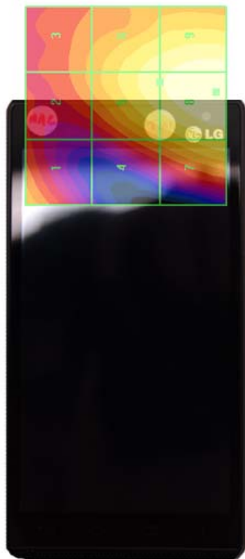
Figure 17-4 E-Field WD Scan overlay
