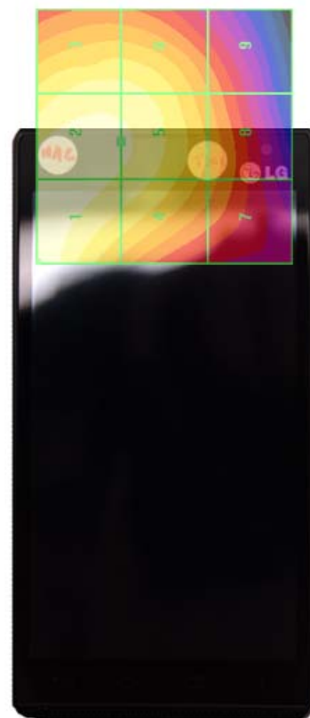
Figure 17-5 H-Field WD Scan overlay
