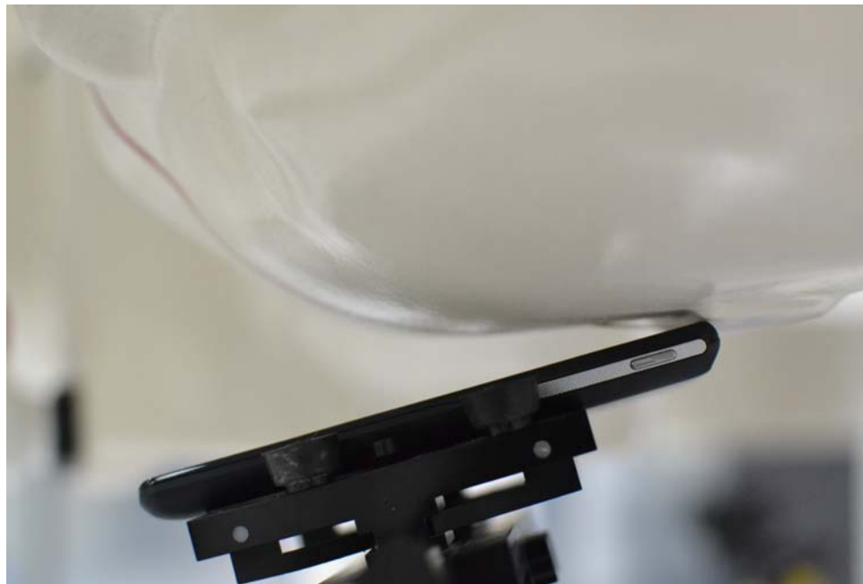
SAR Test Setup Photo 4: Left Tilt
