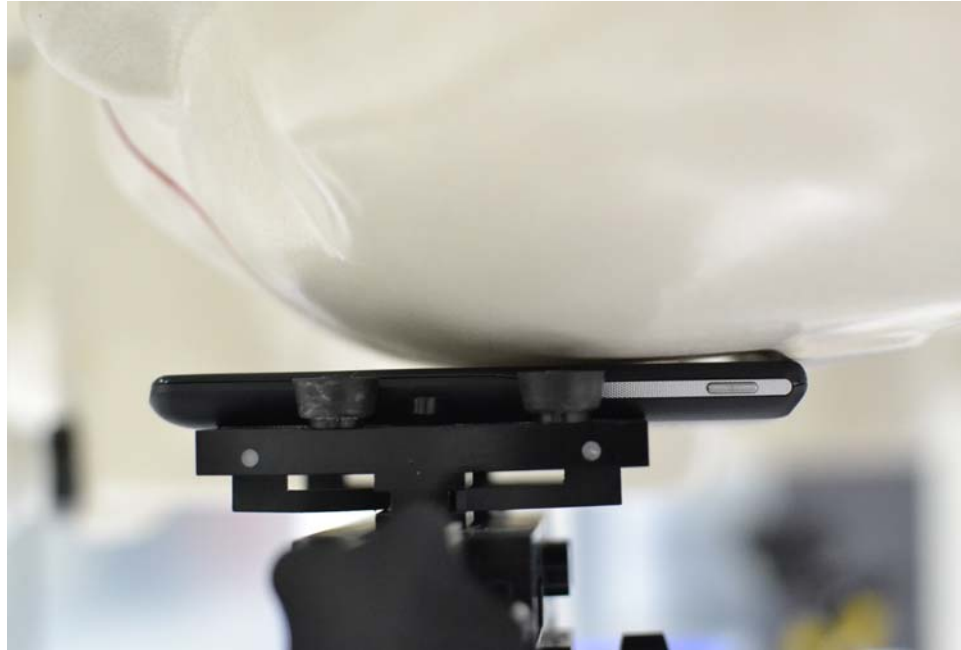
SAR Test Setup Photo 3: Left Cheek
