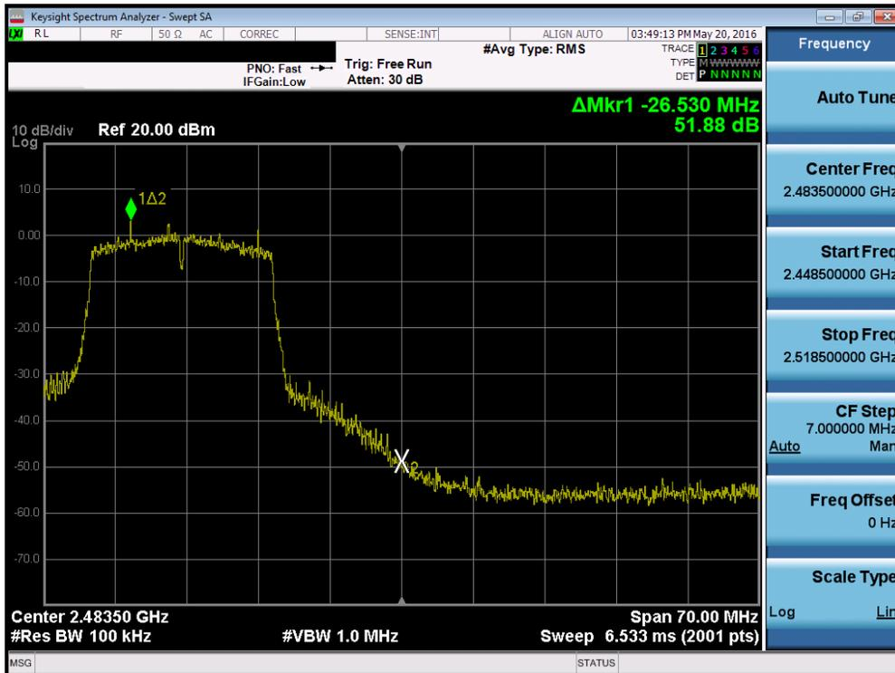
Plot 7-24. Band Edge Plot (802.11n (2.4GHz) – Ch. 11)
