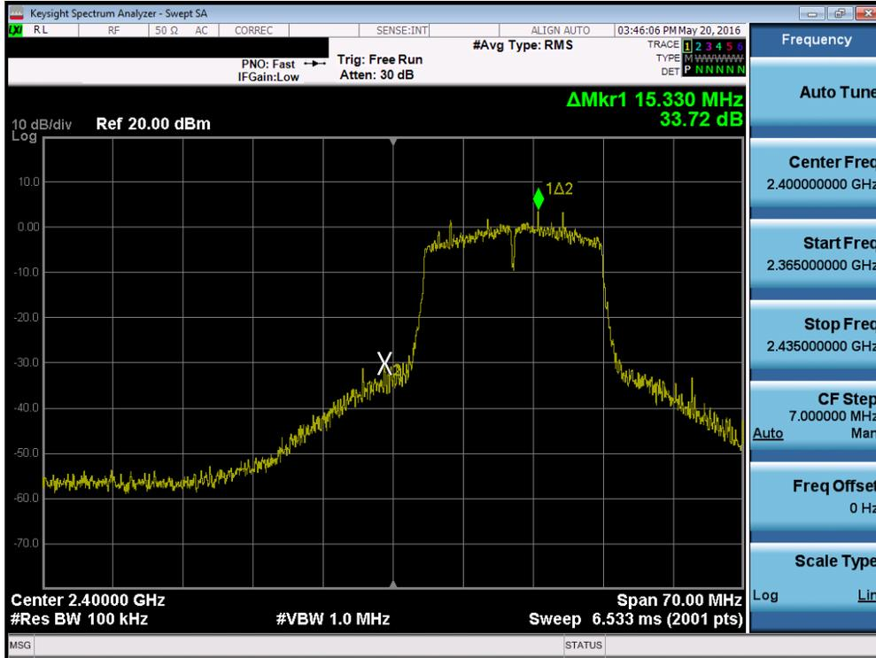
Plot 7-23. Band Edge Plot (802.11n (2.4GHz) – Ch. 1)
