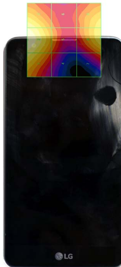
Figure 17-4 E-Field WD Scan overlay
