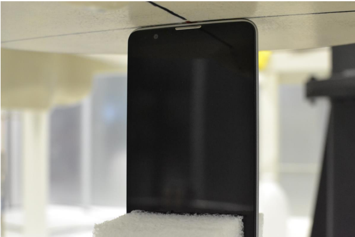
SAR Test Setup Photo 10 – Top Edge at 0 mm
