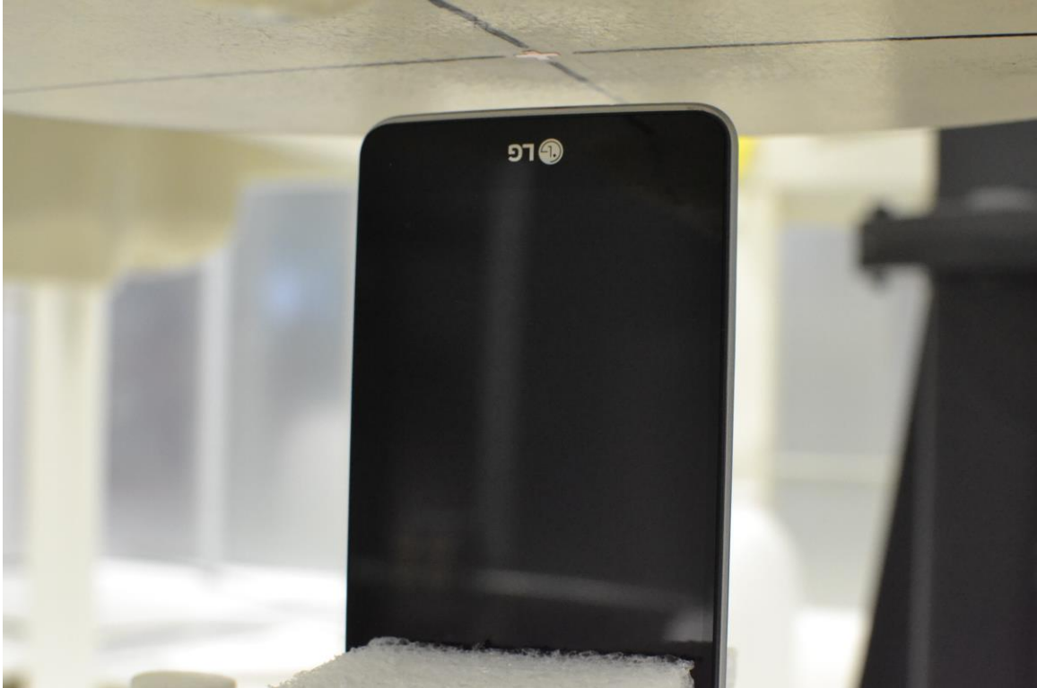
SAR Test Setup Photo 11 – Bottom Edge at 10 mm
