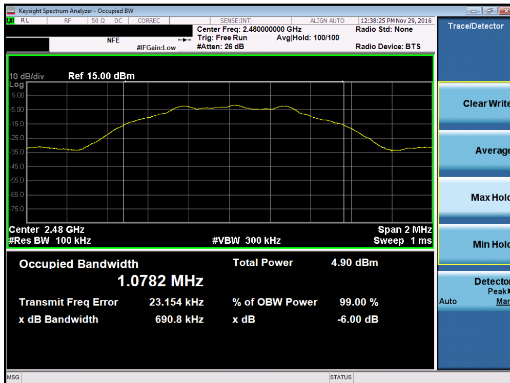
Plot 7-3. 6dB Bandwidth Plot (Bluetooth (LE) – Ch. 39)
